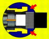
Chamfered edge for ease of cable entry
