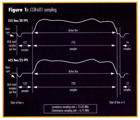
13.5 Msamples/sec and 6.75 Msamples/ sec, well in excess of the NTSC luminance bandwidth of 4.2 MHz and a maximum bandwidth of 1.5 MHz for the
