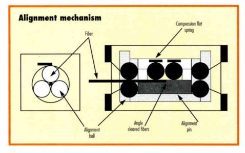
addition to the hi-viscosity index matching liquid in the inner mating chamber, gaskets are used at either end of the device as a sealing barrier to prevent moisture or other contaminants from entering the connection.
