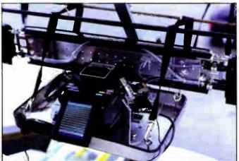
With only a twenty inch taut-sheath opening (cut in the center for no dead fiber in either direction), the FSM-30R12 design gives you at least 3 splice attempts. Try that with a conventional mass fusion splicer!
