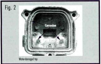
Possible signal level effects from water damage at tap
