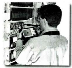
The VFS 1 Video Fiber Scope provides the ability to inspect fiber optic connectors through adapters in patch panels, network elements, and test equipment. For more information on the VFS 1 or our fiber optic test equipment product line visit our web site.
