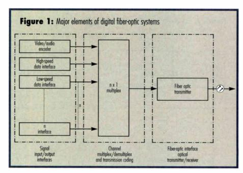
high data rate uncompressed video channels, and each manufacturer's multiplex can be different. Most proprietary systems can implement bi-directional operation but are not required to be symmetrical. Downstream (broadcast) and upstream (reverse) capacity can be tailored to fit specific system needs.
