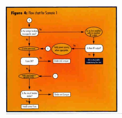
used to energize a specific power path and further determine the bad leg. It also is possible to use an ammeter to measure current and create the continuity. Caution is advised when doing this because the ammeter may have a current limitation of its own.
