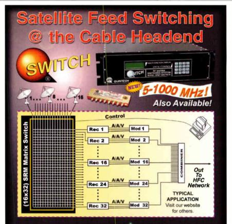
Transparent over the frequency range of 5-1000 MHz (cable) and 950-2150 MHz (satellite), our patented Q-switch products automate the management of broadband RF switching & routing for all advanced telecommunications systems. Our hardware protocol is compatible with all major M & C systems.
