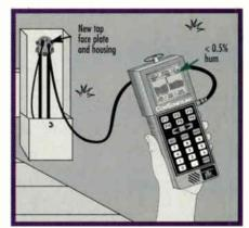
Figure 4: Measuring acceptable hum after replacing tap face plate and housing
