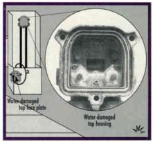
Figure 3: Water-damaged tap causing unacceptable hum
