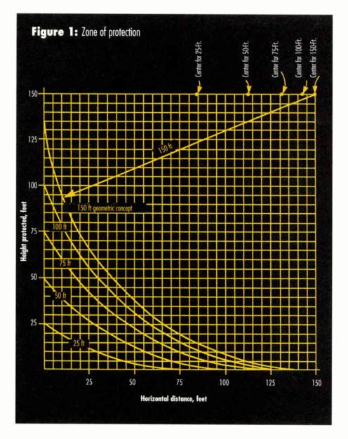
sphere is in the zone of protection. If more than two towers (or lightning rods) are involved, multiple spheres may be used to determine the zone of protection. (See Figure 2 on page 75.)
