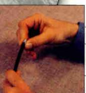
Step 5: If required for the particular connector being used, fold the braid back over the jacket.
