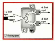
Figure 2: Insertion loss effects of two-way splitters
