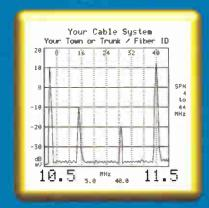
The RDU measures Ingress and Noise, where you designate, by selecting up to 200 frequencies from 4 to 44 MHz. The RDU measurement the analysis and displays RTs acclusive LNAN number.
