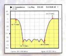
Deletion Filters Channels 2 - 78
