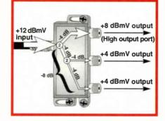
Figure 2: Approximate insertion loss effects of unbalanced three-way splitters
