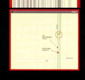
Network management systems can help locate service interruptions fast. By inputting the "length-tofault" distance obtained from an OTDR trace, you can quickly find the fault and display it on a map.
