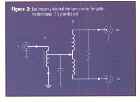
then group engineer with Prime Cable, wrote about this in an article that appeared in the May 1990 issue of *Communications Technology* ("Hum Modulation in Drop Passives," page 28). Hepler's focus was how this problem affected addressable converter data carriers in one-way systems. His article described an example where a voltage drop of just 3 V across a neutral conductor
