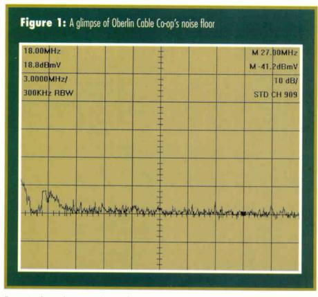
Figure 1: The total return path noise floor of Oberlin Cable Co-op's entire system, including approximately 120 trunk amps and line extenders with about 2,000 filtered drops into the hub, which feed input to the LANCity headend controller.
