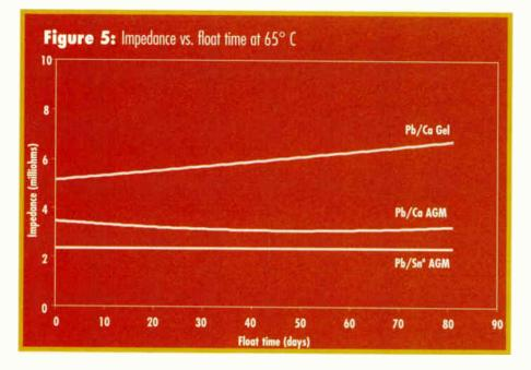
impedance of 2.4 milliohms and never increased. The lead-calcium AGM battery started with 3.5 milliohms and remained constant. The gel cell battery started at 5.2 milliohms and increased to 6.7 milliohms on day 80. The lead-tin battery's lower impedance allows it to discharge energy faster and recharge faster.
