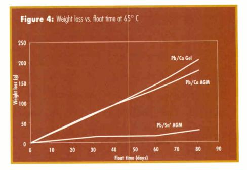
ing an 80-day float period at 2.27 V per cell and 65° C. The lead-tin battery lost 29 grams. The lead-calcium AGM battery lost more than six times that, 179 grams, and the gel cell lost 205 grams.
