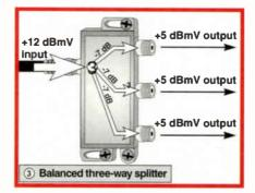
Figure 1: Approximate insertion loss effects of balanced three-way splitters
