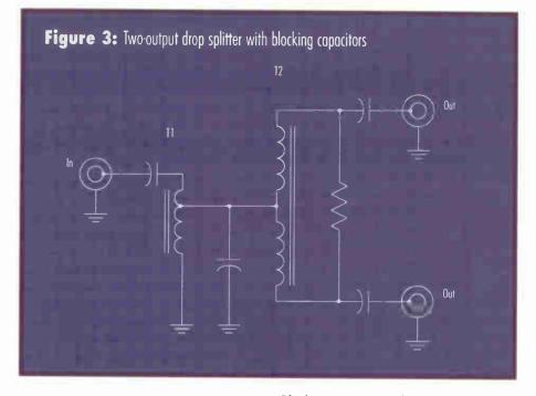
could produce a current flow of 5.53 amperes on a drop, 17 percent of which would appear on the center conductor. That's 0.94 ampere, clearly enough to saturate a drop splitter's tiny ferrites.
