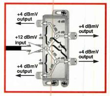
Figure 3: Approximate insertion loss effects of four-way splitters
