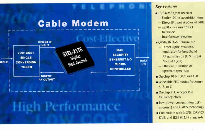
Combine our STEL-2176 Digital Modulator/Demodulator ASIC with a simple tuner and a single controller ASIC and you have ... the highest performance, competitively priced, worldwide standards compatible subscriber modem solution available today.
