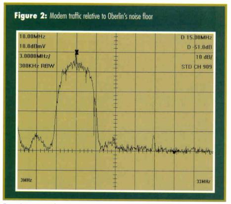
Figure 2: Represents identical conditions with Zenith cable modem traffic depicted relative to the noise floor indicating the relationship between the traffic and the noise floor. Because Oberlin's setup uses Zenith gear for schools and municipal government intranet, and LANcity equipment for its Internet subscriber platform, it is a very flexible hybrid data solution, says Poge Smit.
