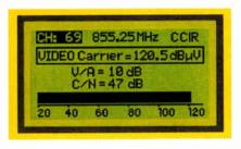
possibility to measure the signal LEVEL of the video carrier, the VIDEO / AUDIO RATIO or the CARRIER / NOISE RATIO. It is possible to choose what measurements we want to carry out (carrier level or level + V/A + C/N) so as not to waste time, for
