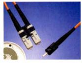
The Methode ST⊕ and SC Quick Cure™ system combines patented polymer ferrule technology with a rapid cure adhesive. The pedestal tip reduces fiber breakage, and the 20 second curing interval decrease field termination procedure time.
