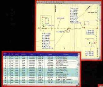
Cable engineers can now use computer tools to give them access to a variety of physical plant data including: fiber routes, cable lengths, cable type and count, splice type and location, and loss values.
