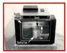
Figure 4: Picture effects of too high input signal to amplifier
