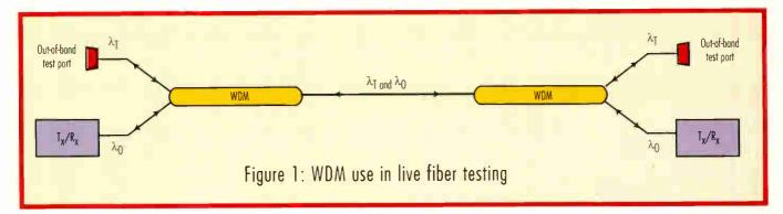
shown in Figure 1, where  $\lambda_0$  is the operating wavelength and  $\lambda_T$  is the test wavelength from the OTDR. It is important to put WDMs at both ends of the link to prevent  $\lambda_{T}$  from reaching the receiver. This also allows the OTDR to be connected to either end of the link for bidirectional testing.
