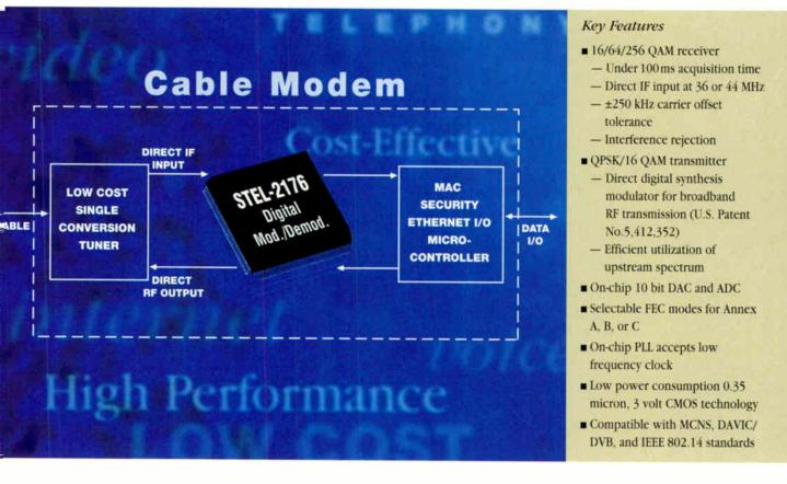
Combine our STEL-2176 Digital Modulator/Demodulator ASIC with a simple tuner and a single controller ASIC and you have . . . the highest performance, competitively priced, worldwide standards compatible subscriber modem solution available today.
