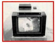
Figure 3: Picture effects of too low input signal to amplifier
