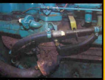
A periodic inspection of all hoses is in order. Check for pliability, cracks, leaks and weak spots.
