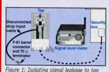
Figure 1: Isolating signal leakage to tap by disconnecting service drop from tap
