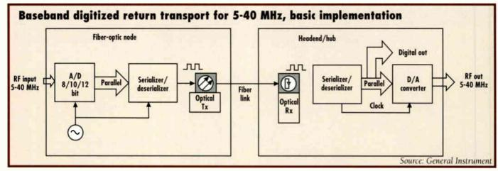
and then transports it to the headend via fiber as a digital signal. The reverse spectrum is digitized using high-speed analog-to-digital (A/D) converters, which currently can sample 10 to 12 bits at 100 or more MHz samples per second (MSPS), and then returned to the original 5-40 MHz spectrum at the headend using a digital-to-analog converter (D/A). (See the accompanying figure.) Time division multiplexers can be employed at the node to combine several digitized return spectra onto one fiber.
