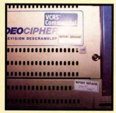
Keep track of battery replacement by labeling equipment with the date the battery was installed.
