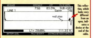
The top waveform shows a substantial upward reflection, which indicates a complete open (nothing reflected on the cable). This would indicate that the cable is not connected to a device such as a TV set or VCR. The bottom waveform is dissimilar from the first in that it indicates that a device is connected to the cable and that service theft could be occurring.
