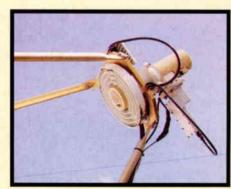
Even a small hole as seen in the lower part of this feedhorn screen can cause maintenance headaches. Carefully inspect the entire satellite dish for damage.
