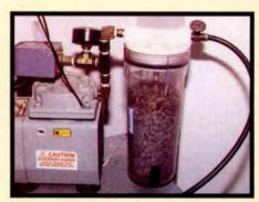
Make sure your dehydrator crystals are blue indicating that the line gas is dry. Even a canister with half blue and half pink crystals is better than no moisture absorption at all.
