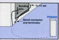
Figure 3: Terminating drop cable at ground block
