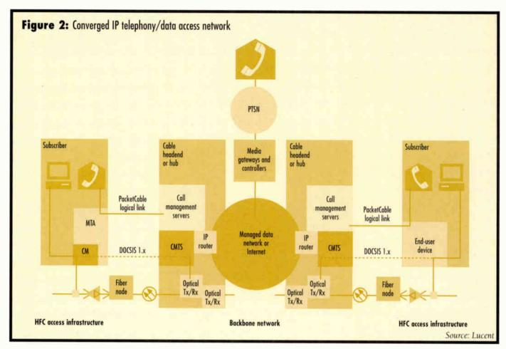
Integrating IP telephony networks with high-speed data services, using common transport equipment both at the headend and an integrated end-user device at the customer location, saves money and increases efficiency in local and backbone transport.
