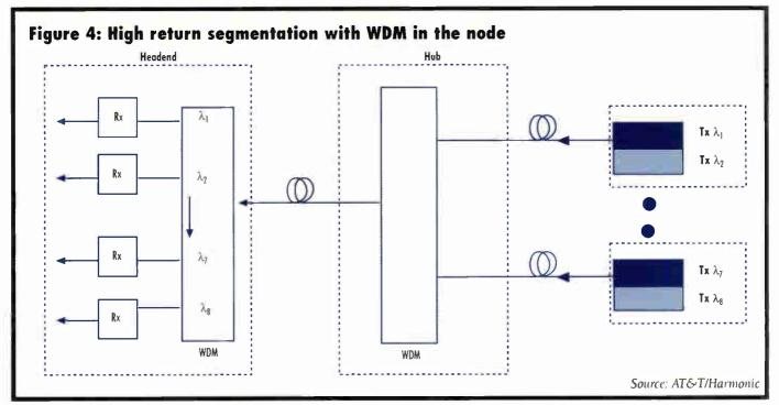
Implementation of DWDM transport networks for AT&T B&IS systems falls into two broad categories. The first category covers those systems where only highspeed Internet access services are deployed initially. In these systems, the segmented service areas support a full narrowcast lineup but utilize only a portion of it.
