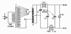
WHILE there are still many homes not supplied by electricity, by far the majority of those in which radio receivers are operated are wired for 110-volt, 60 cycle A. C. current suitable for operating a receiver with the necessary apparatus to change the A. C. current into the required values of direct current for the operation of a receiver.
