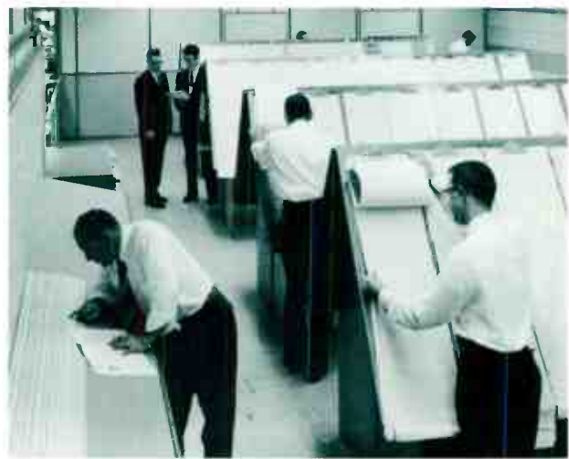
The display room where hundreds of feet of chart paper record each Bomarc flight.
