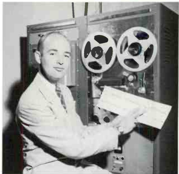
Dr. Robert Helliwell points to trace from a recording made on whistler-detecting equipment shown behind him. Peaks in upper curve represent whistlers; height of peak indicates relative amplitude. Lower curve is corresponding frequency distribution.
