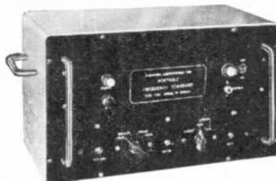
Frequency Standard—1744 —1 kc/s to 80 Mc/s—0.005% accuracy.
