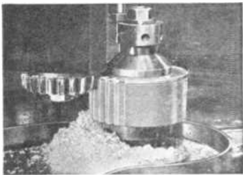
Tufnol is easily machinable with ordinary workshop facilities. Photograph shows a Tufnol gear being cut.
