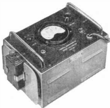
Diode Voltmeter—281C/2 —50 c/s to 250 Mc/s, 0.1V to 150V a.c.—0.2 to 300V d.c.
