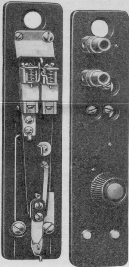
The two strings, which are made of 0.4 mil tungsten wire, as in the case of the single string element, are insulated from each other electrically so that they may be used to observe simultaneously any two different electrical phenomena. An example of this would be to show the phase difference between currents and voltages in different or the same parts of a circuit and so forth. One string may be vibrated at a known frequency to serve as a timing element for the other string.
