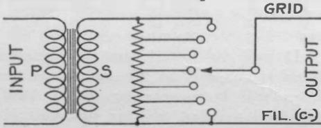
This device makes an excellent and thoroughly reliable gain control for a speech amplifier when used in the manner suggested in the diagram.
