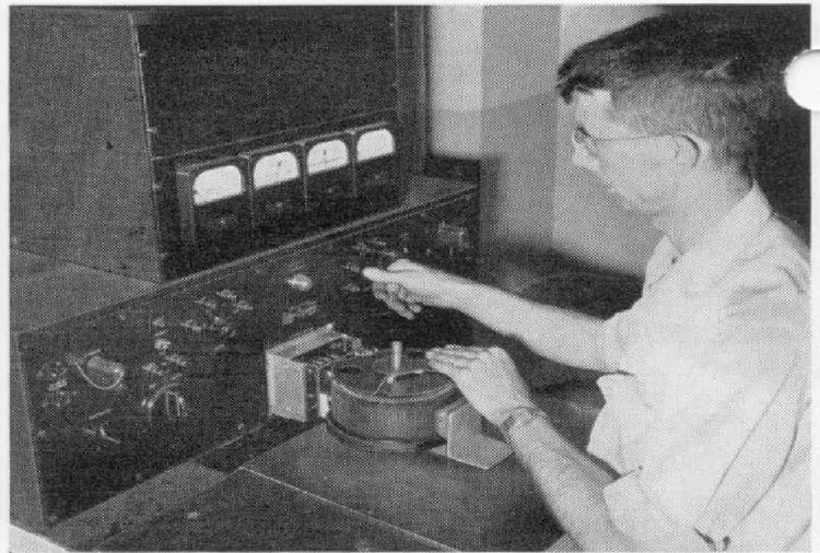
Prior to shipment, all Variacs must pass a series of rigid electrical tests to assure conformance to specifications.
