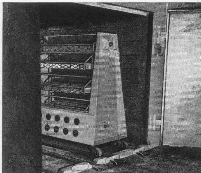
Rack, with load of Variacs, then goes into an oven to bake the thermosetting varnish.
