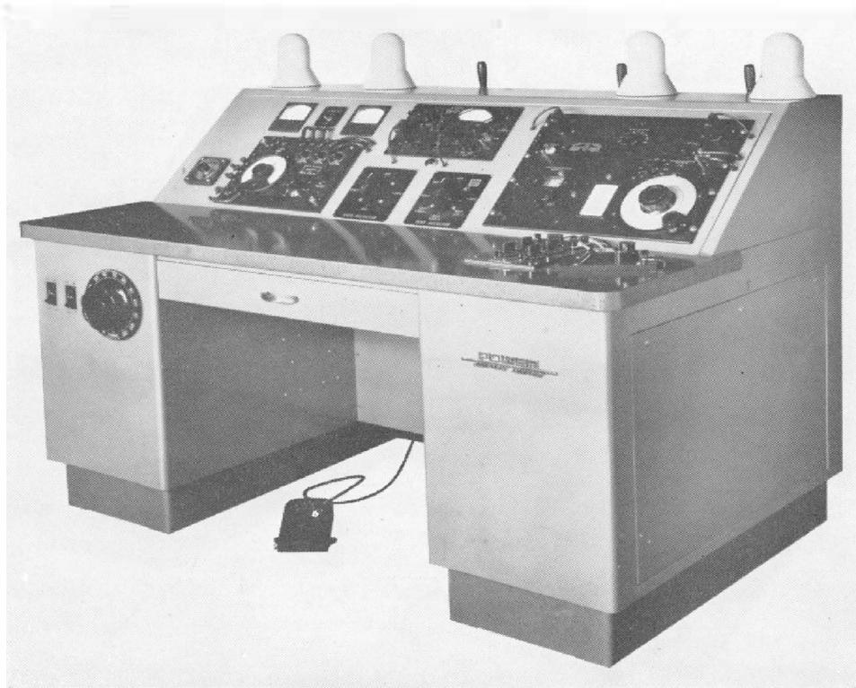
Figure 1. View of the console for preliminary electrical tests. The Type 716-C Capacitance Bridge is at the right, the Type 1231-B Amplifier and Null Detector at the top center of the pouch. At the left part of the console is the Variac® Autotransformer.
