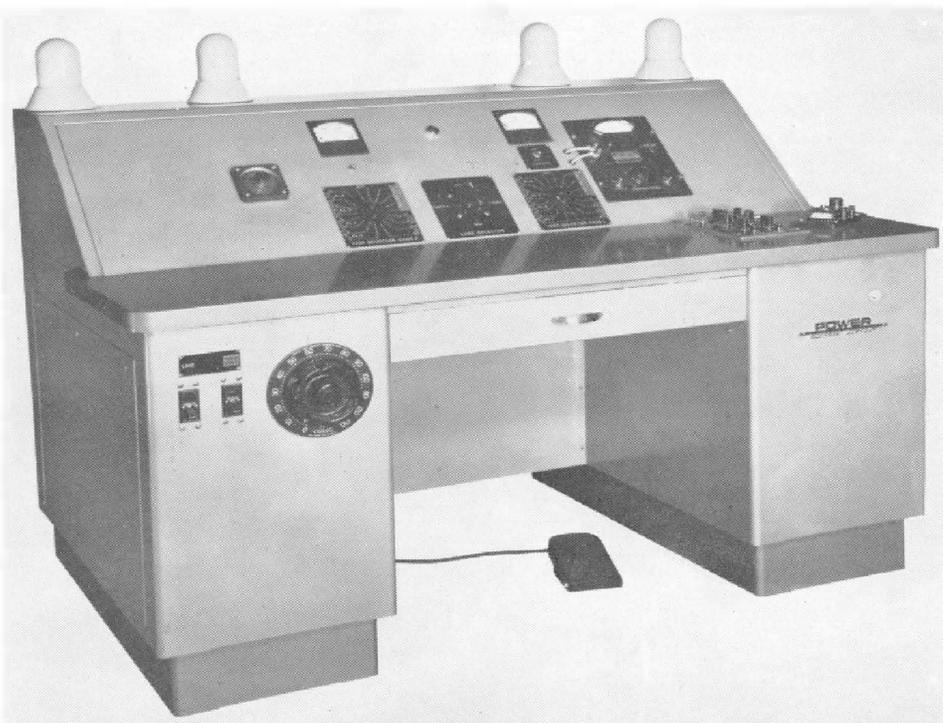
Figure 2. View of the console for final electrical tests. The General Radio Megohmmeter is at the right of the panel, and the Variac at the front face of the left-hand pedestal.
