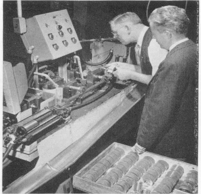
Figure 3. Designed and built in General Radio's tool department, this machine automatically mills the rotors and stators from the aluminum extrusions shown in Figure 4.
