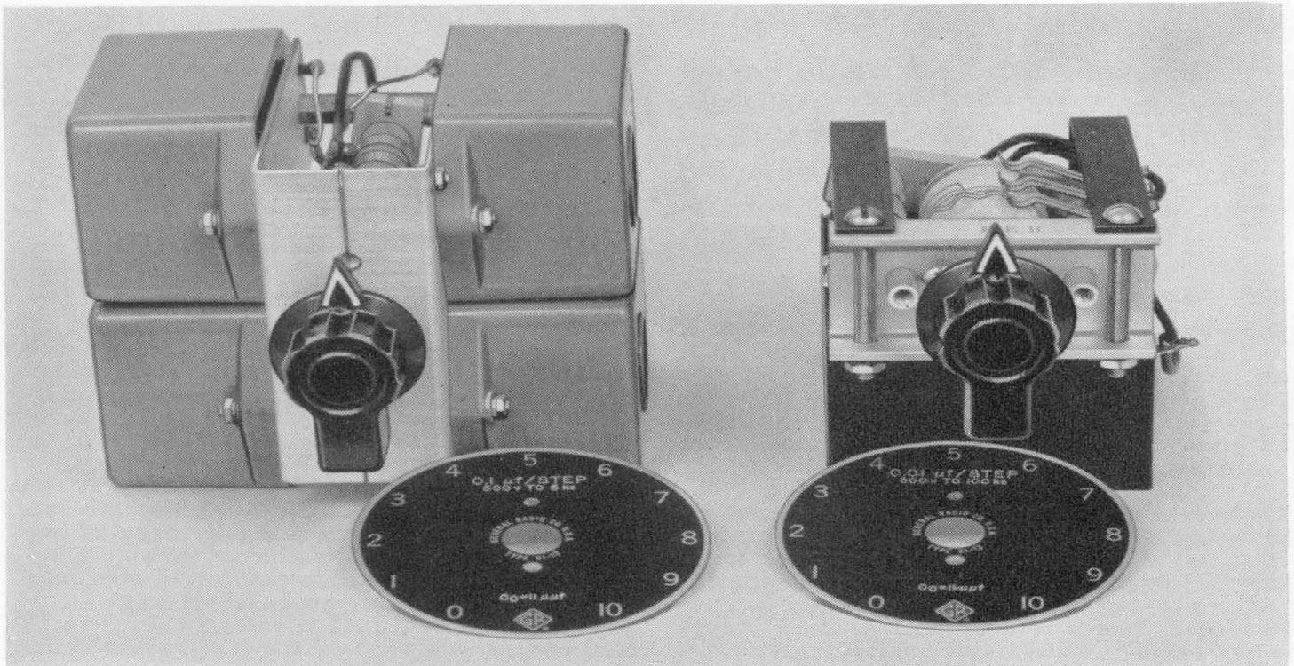
View of the Type 980-F (left) and Type 980-N (right) Decade Capacitor Units.
