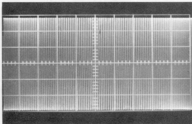
Figures 4a (left) and 4b (right). Waveforms produced in the same manner as those in Figure 3, except that the driving signal is a continuous one of (a) 2.95 kc. and (b) 3.0 kc. The variation of amplitude indicates the presence of standing waves, which obscure the transducer's frequency characteristic.
