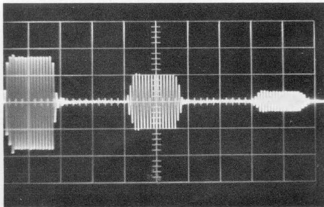
Figures 3a (left) and 3b (right). Waveforms received by one of two transducers mounted in the end of a closed tube, when the other transducer is driven by a tone burst of (a) 2.95 kc. and (b) 3.0 kc. From left to right, the pulses are the direct response, the first reflection from the tube end, and the second reflection from the tube end. Notice the consistency in amplitude of the direct pulse at the two frequencies; compare with Figures 4a and 4b.
