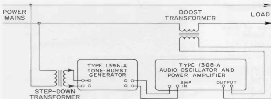
Figure 7. Tone-burst system for generating power-line transients.
