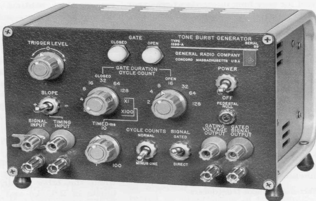
Figure 2. View of the Type 1396-A Tone-Burst Generator.
