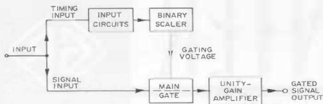
**Figure 1. Elementary block diagram of the Type 1396-A Tone-Burst Generator.**
