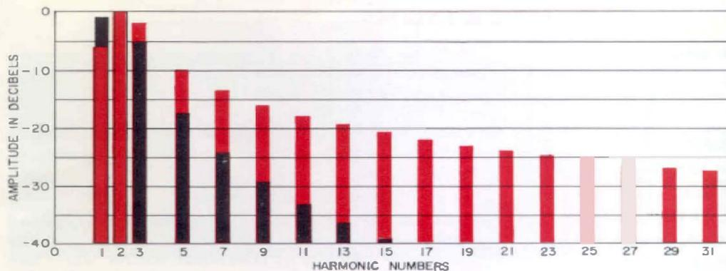
Figure 8. Amplitude of the first 31 Fourier harmonics of a one-cycle-on, one-cycle-off tone burst. Switching at zero crossings in black; switching at peak points in red.
