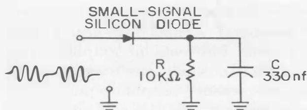
Figure 5a. Example of a simple rectifying circuit tested with a tone burst.
