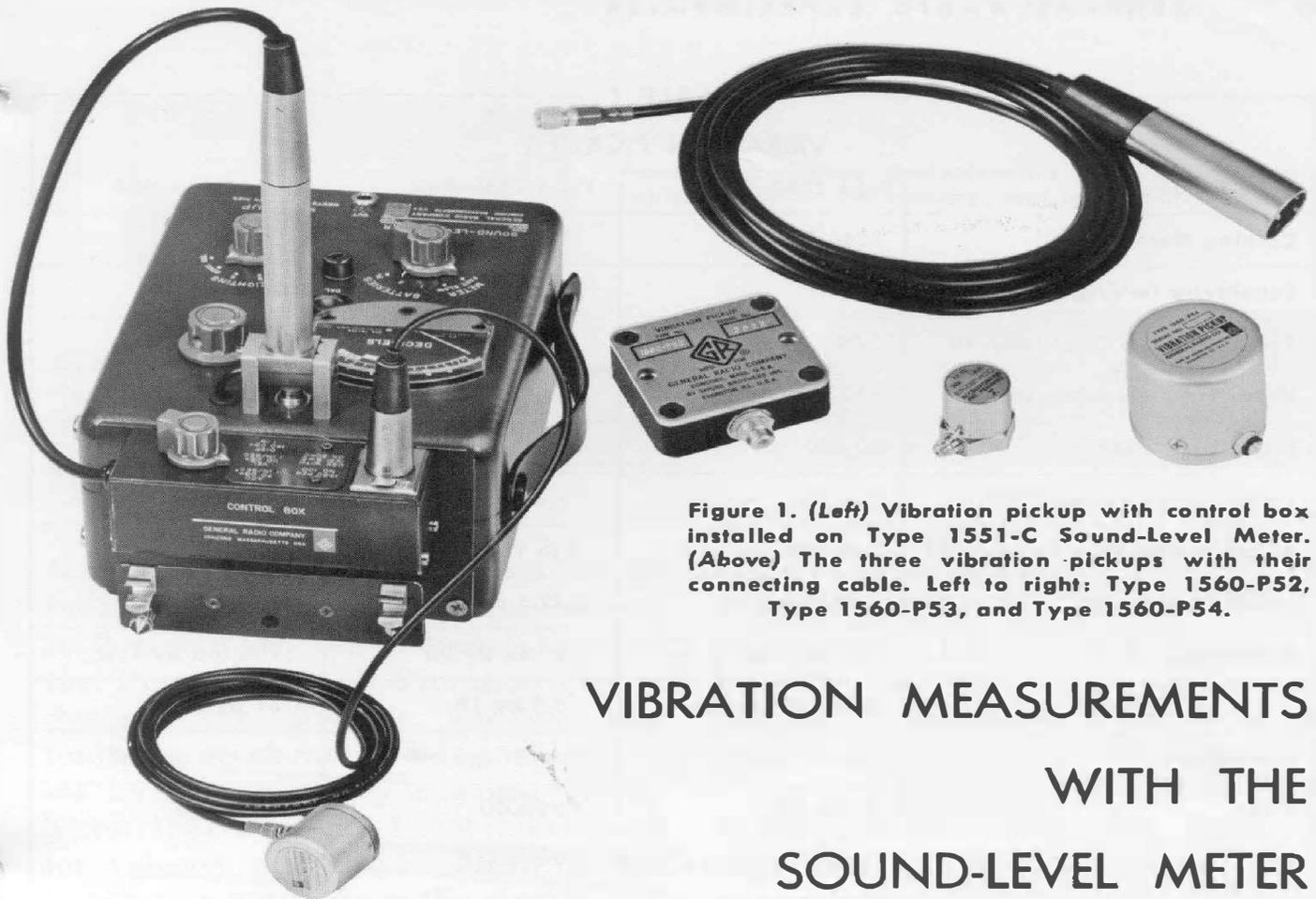
Figure 1. (Left) Vibration pickup with control box installed on Type 1551-C Sound-Level Meter. (Above) The three vibration pickups with their connecting cable. Left to right: Type 1560-P52, Type 1560-P53, and Type 1560-P54.
