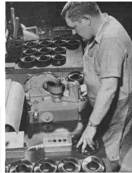
To speed production on the thousands of control knobs that go into GR instruments, the semi-automatic machine shown at left bores, drills, counterbores, taps, and inserts setscrews into each knob.
