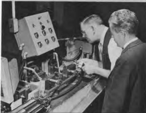
The coils for Variac® autotransformers are wound on the GR-designed machine, shown above, which applies an evenly spaced winding, accurately banked on the inner face, to the toroidally shaped core.
