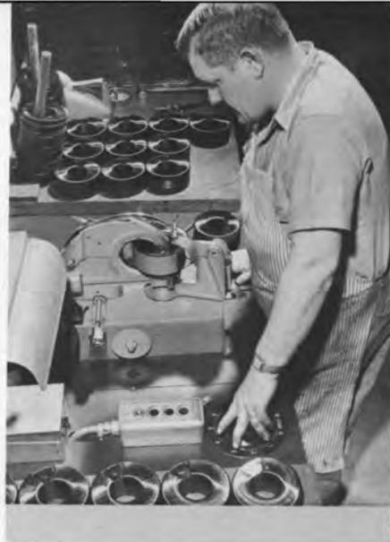
To speed production on the thousands of control knobs that go into GR instruments, the semi-automatic machine shown at left bores, drills, counterbores, taps, and inserts setscrews into each knob.
