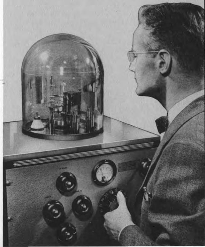
A continuous program of standardization of resistance, inductance and capacitance is carried on in the Standardizing Laboratory, whose determinations are checked periodically with the National Bureau of Standards. Here, also the electrical properties of new materials appearing on the market are measured. The Engineering Staff uses this laboratory for critical measurements in connection with instrument development.
