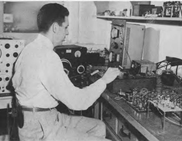
*Development engineering starts with the "breadboard" models on which the basic circuit, components and performance characteristics are determined.* ←
