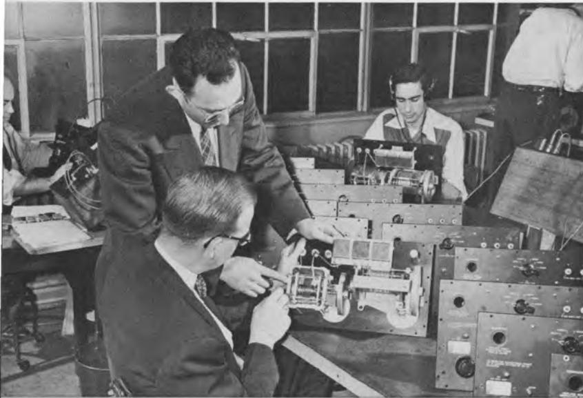
The safety of airline passengers and the success of military operations may depend upon the accurate calibration of these aircraft fuel-tank-gage testers.
