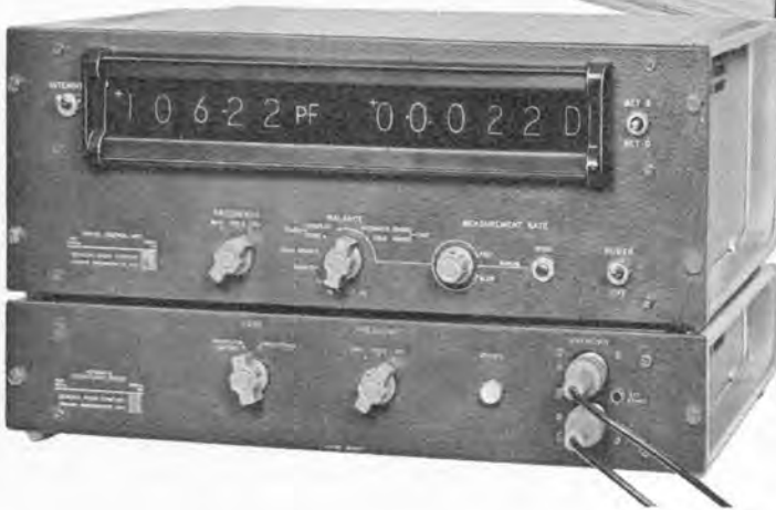
(Above) The Type 216 Capacity Bridge (1921), for many years the industry standard; (left) the Type 1680-A Automatic Capacitance Bridge, newest of General Radio's extensive line of bridges.
