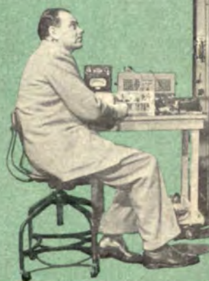
→ Two Parts in 100 Million is the accuracy of this primary-frequency standard, the result of 30 years of continuous G-R development. One of these instruments, a standard catalog item, supplies frequencies throughout the Cambridge plant.
