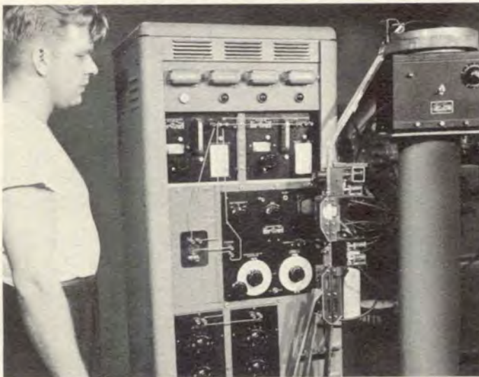
Automatic Sorting of capacitors is accomplished using a General Radio Impedance Comparator and auxiliary GR Precision Capacitors and Decade Resistors. This instrument's circuits are designed to facilitate automatic control techniques and recording. GR equipment is designed with an eye to the future.
