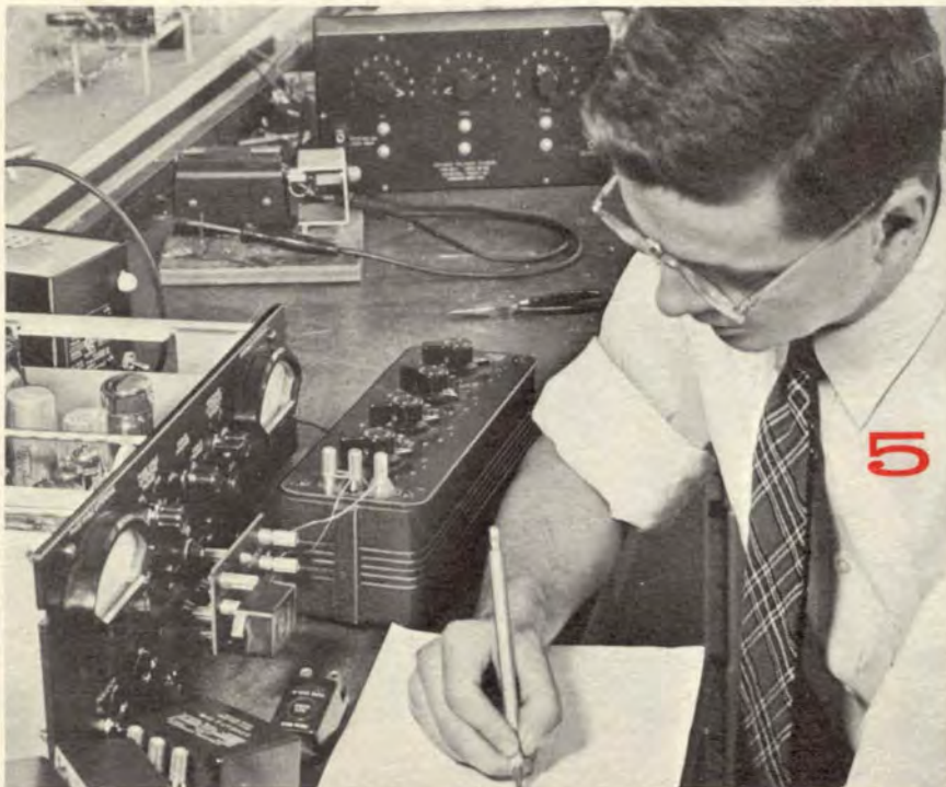
Development Engineer Tests Prototype with aid of standard resistors and capacitors to see how the new design performs in the finished package. When these tests are concluded, most mechanical and electrical problems will have been solved.
