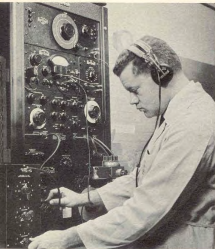
Laboratory Investigations with precision G-R Capacitance Measuring Assembly take the guesswork out of plastics. Electrical properties of new resins are studied to gain additional insight into the physical compositions of these materials. Both dielectric constant and dissipation factor are determined with a high degree of accuracy.
