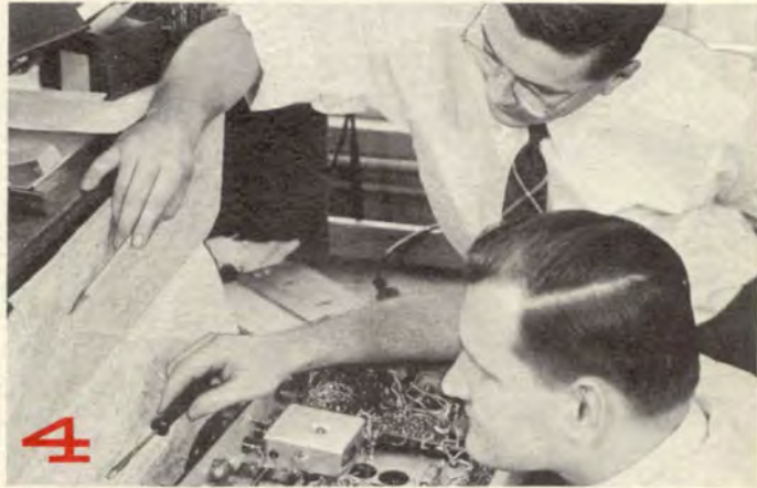
Prototype Is Built by expert technicians and machinists in the Experimental Shop. Above, a technician, working from a circuit diagram, is mounting components on a panel that was made by the machinists from drafting sketches.
