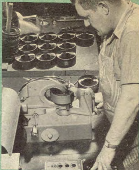
→ Coils For Variac® autotransformers are wound on this unique GR-designed machine, which applies an evenly spaced winding, accurately banked on the inner face, to the toroidally shaped core.
