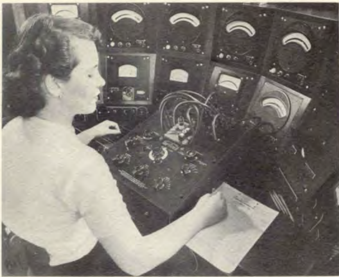
Electron Tube Manufacturer Uses GR Vacuum-Tube Bridge as standard to calibrate all the other tube checkers in his plant. Wide ranges of tube and transistor dynamic characteristics are measured with high accuracy using this precision bridge.
