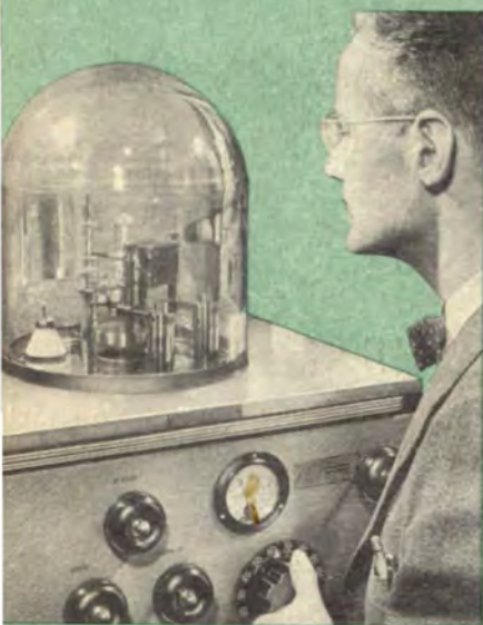
← Quartz Crystals are manufactured at GR on an individual basis in the laboratory. This assures the stability required for use in GR primary frequency standards and GR broadcast station frequency monitors.
