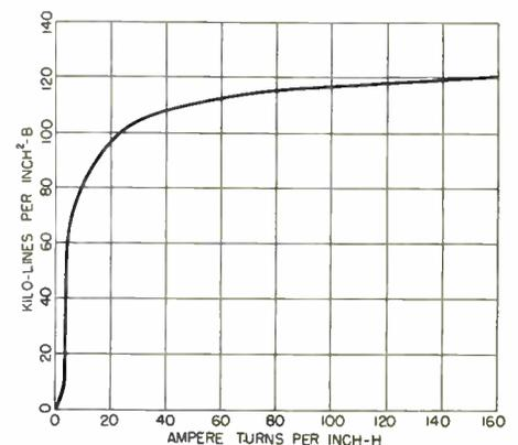
**Figure 5—A B-H curve for a sample of silicon steel, indicating permeability and effect of magnetic saturation.**
