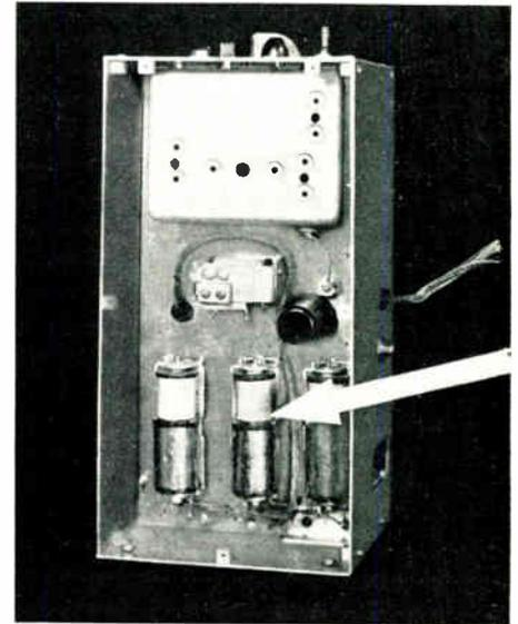
Figure 6—Rear view, cover removed. Arrow points to center slow-release relay.
