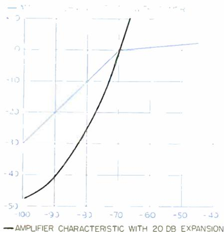
Figure 1—Blue curves represent typical response of peak limiter compressor. Black curves represent typical response for volume expander.
