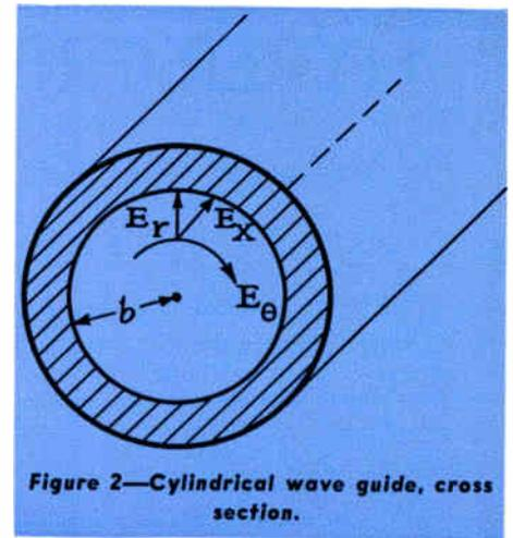
Figure 2—Cylindrical wave guide, cross section.
