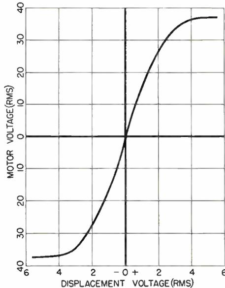
Figure 8—Curve representing a-c voltage supplied to the variable, phase winding of motor as a function of displacement voltages resulting from errors in clockwise and counter-clockwise directions.
