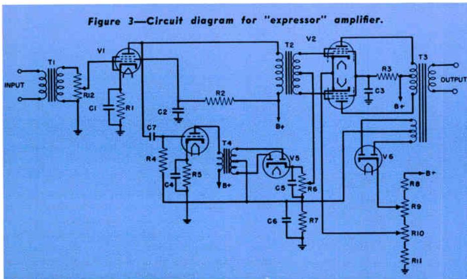
Figure 3—Circuit diagram for "expressor" amplifier.
