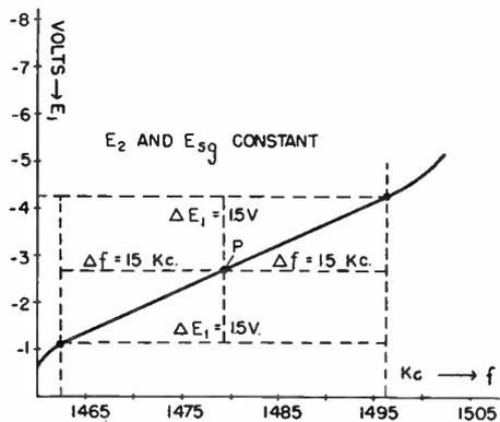
**Graph showing frequency as a function of the positive voltage applied to the accelerating grid.**
