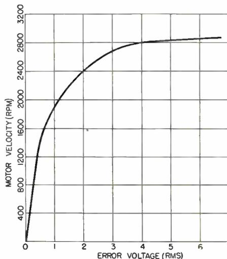
Figure 9—Curve showing motor velocity for different a-c voltages applied to variable phase winding with 75 volts across the fixed phase winding. Voltage across latter winding lags the control voltage by approximately 90°.
