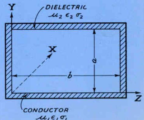
These waves are characterized by the presence or absence of the component of electric intensity or magnetic intensity in the direction of propagation. They are known as transverse electric waves (TE) denoting the absence of the component of electric intensity in the direction of propagation or transverse magnetic waves (TM) denoting the absence of the component of magnetic intensity in the direction of propagation.
