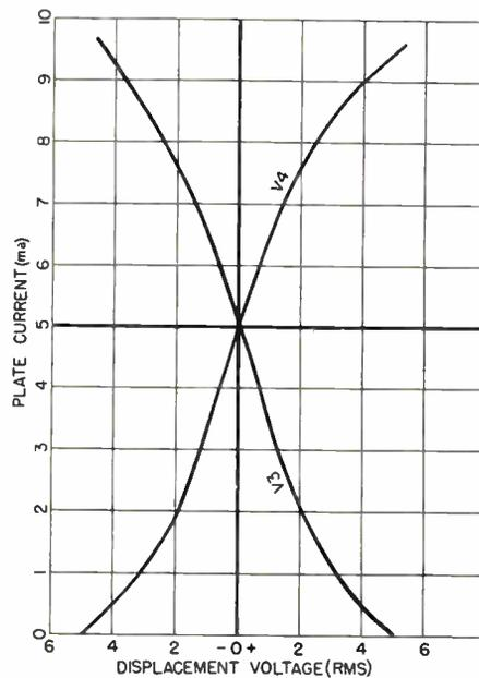
**Figure 4—Curves showing variations in plate current in each half of the amplifier tube for different displacement voltages of each phase.**
