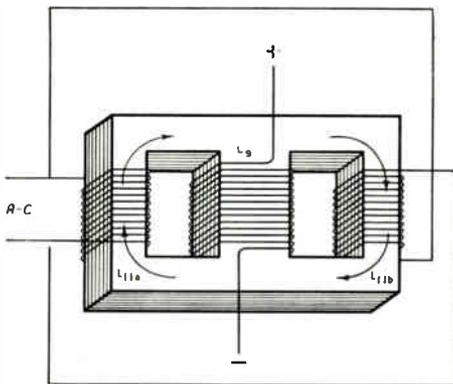
Figure 7—Manner in which windings are placed on the core of a saturable reactor.
