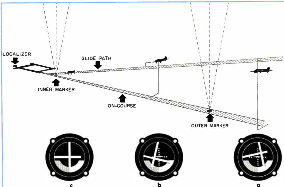
Figure 4—Diagram of glide path and markers showing position of visual indicators when (a) low and to the left (b) high and to the right, and (c) on course.
