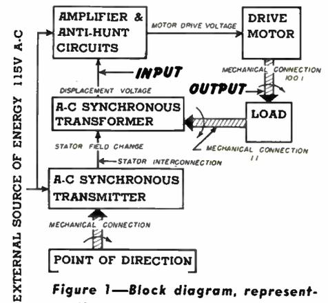
Figure 1—Block diagram, representative of most electronic servos.
