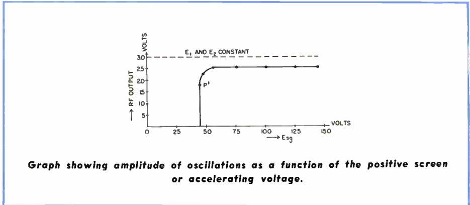
**Graph showing amplitude of oscillations as a function of the positive screen or accelerating voltage.**
