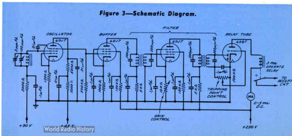
Figure 3—Schematic Diagram.
