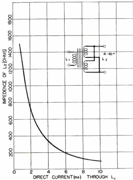
Figure 6—Curve representing impedance of each reactor as a function of a direct current flow in the control winding.
