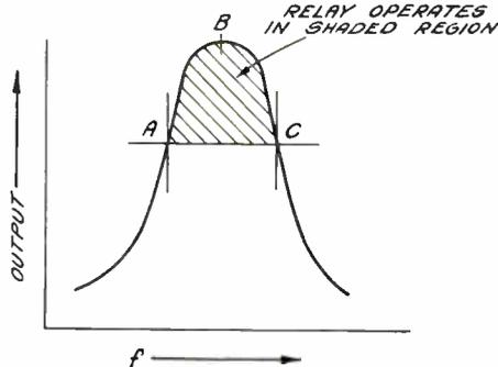
Figure 2—Overall selectivity curve as filter unit.
