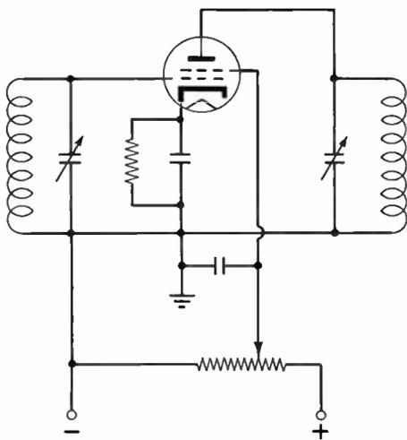
**Circuit diagram of discharge tube oscillator.**
