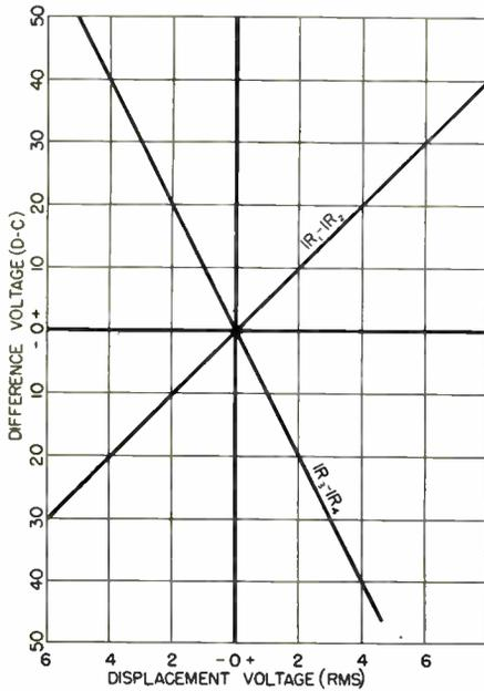
**Figure 3—Curves showing difference between rectified potentials across R1 and R2, and across R3 and R4 as a function of displacement voltages in either phase for small angular displacements.**
