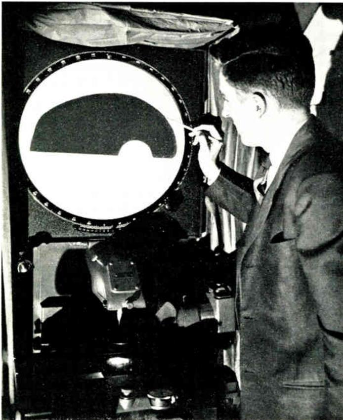
**Contour measuring projector in Mechanical Engineering showing magnified profile of rotor plate.**
