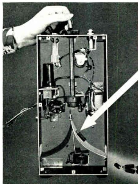
Figure 5—Front view, cover removed, showing rejected core.
