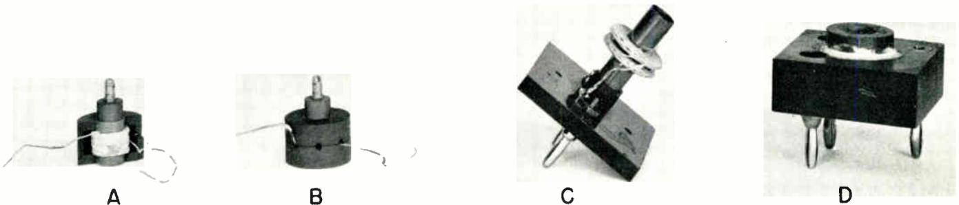
Figure 1—A. Cut-away view of, B, complete coil assembly. C. First test coil found unsatisfactory because of open construction. D. Test jig that has proved to be satisfactory. Readings check to within 0.1% between jigs.
