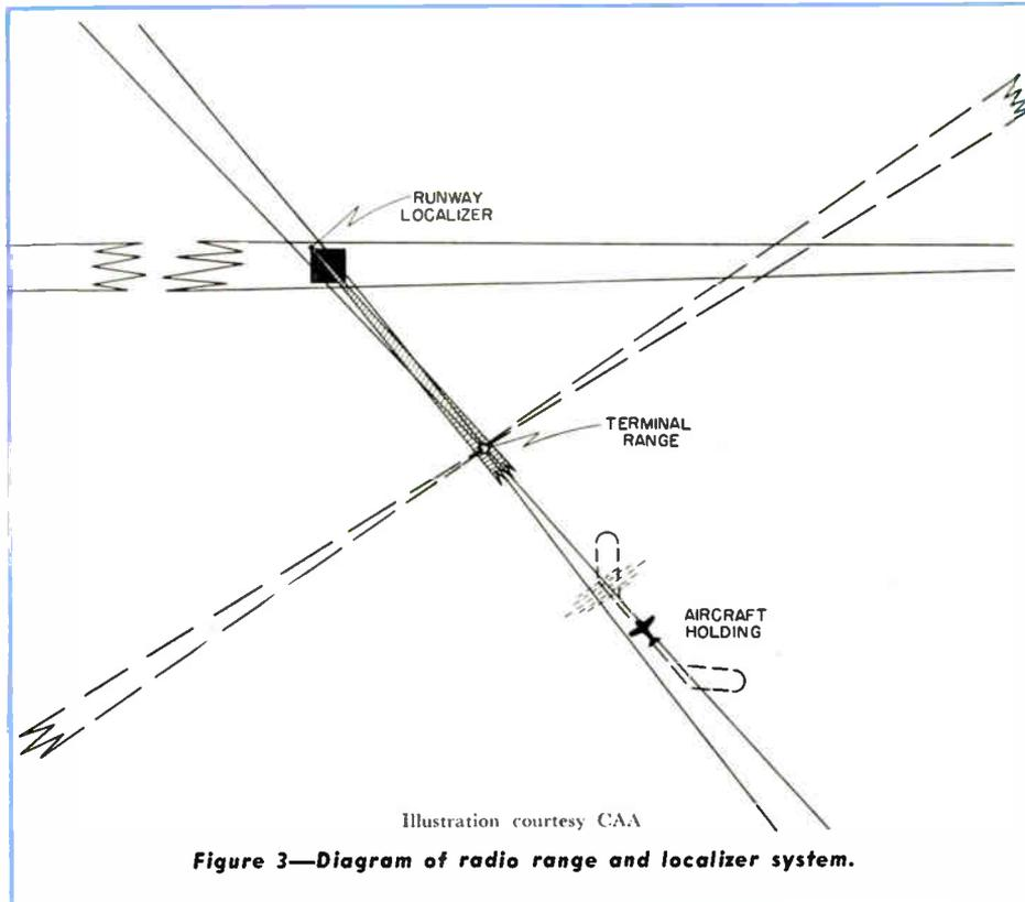
Figure 3—Diagram of radio range and localizer system.
