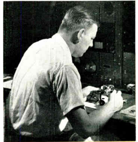
After grinding the quartz blank on glass and abrasive, Leo Servary measures its thickness on a precision micrometer.
