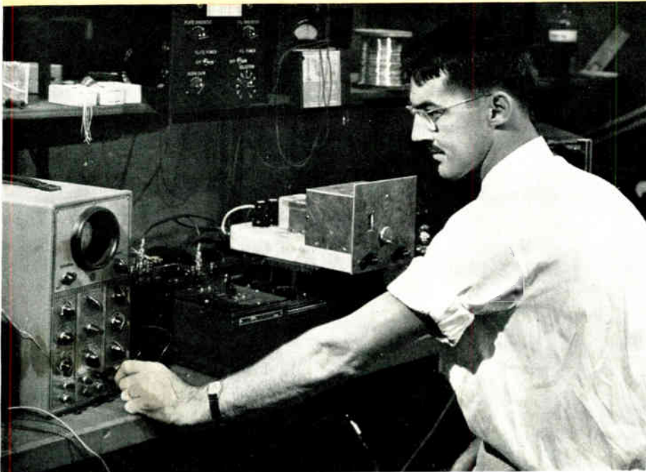
G. R. White, engineer in charge of the development of the wide-band phase-meter, tests the inherent phase shift appearing in the radio frequency converter section.
