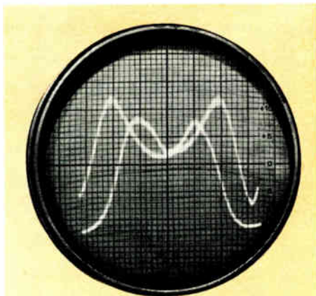
Figure 1—Response curve of an over-all i-f system checked on a cathode-ray oscilloscope shows inaccuracy despite careful alignment by a signal generator with a modulated oscillator.
