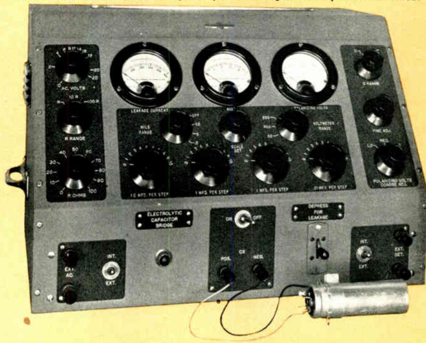
Figure 1—Front view of electrolytic capacitor bridge, with capacitor attached.
