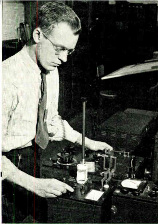
Dielectric properties being measured on a General Radio 516-C R-F Bridge. Thomas Wild, who is operating the instrument, made modifications which permit use of the bridge for computing power factors from 1 kilocycle to 1 megacycle.
