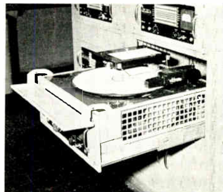
Open drawer of Memovox machine used to make a permanent record of all programs as they go over the air. Recording continues, automatically shifting from one drawer to the other until the program is over.
