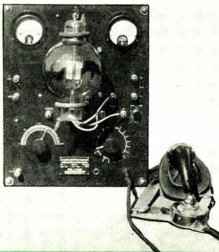
In early 1917, first spoken message from plane to ground in the United States came from this transmitter built by E. J. Simon according to specifications of Captain C. C. Culver, Signal Corps.
