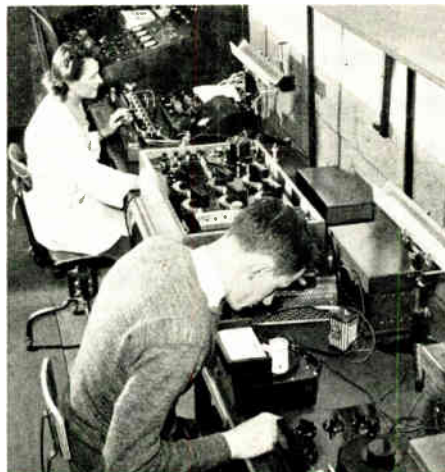
Arborette Feehan, left, watches a mirror-reflected beam of light move across the scale in making resistance measurements with the Leeds and Northrup Kelvin bridge. John O'Gorman, right, checks the calibration of a meter with a Leeds K-2 Potentiometer.
