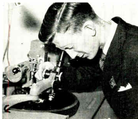
Operator uses microscope to check groove made by recording lathe.
