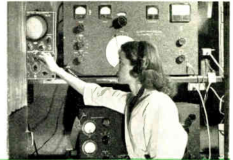
A precision meter is checked with a Brooks Potentiometer by Arborette Feehan, left, and Mary Haynes, right.
