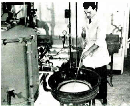
Chemicals for phosphorescent covering of cathode-ray screen are mixed in a steam-heated glass-lined kettle. To keep the ingredients absolutely pure, distilled water from the large tank (left) is used, and dust is removed from the atmosphere by electrostatic precipitation.
