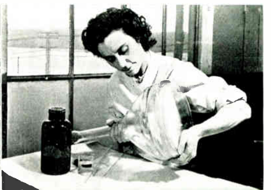
With a circular motion, the worker distributes phosphorescent powder over the inner face of the tube which has been coated with a liquid adhesive. Choice of chemical determines color, persistence, and other characteristics of the finished tube.
