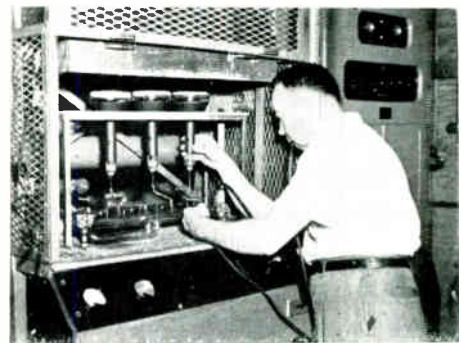
A flat-faced, 5-inch model of cathode ray tube is sealed to the exhaust manifold. The mouthpiece and hose permit control of air pressure in the glass tubing while the dual-burner is manipulated to make the seal.
