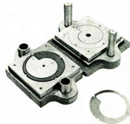
Figure 6—Tool for producing stator plates.
