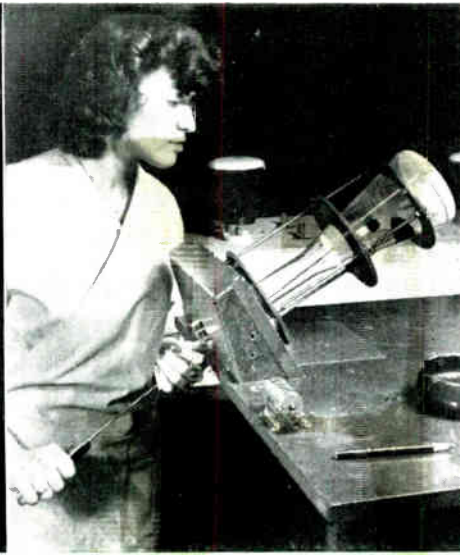
Close-up showing application of black aquadag coating to the side of the envelope. As the jig revolves, the operator manipulates a brush with a long wire handle.
