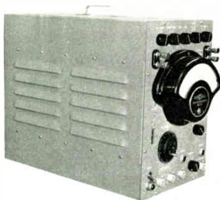
Figure 1—Direct reading, wide band phase and frequency meter.
