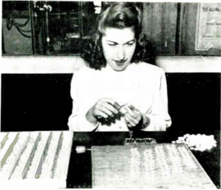
Operator inserts tiny cathodes in a ceramic disc for cathode-ray tubes. From this white tipped cathode is fired a stream of electrons at the phosphorescent screen. A short length of wire is then attached and terminated in one of the tube stem supports.
