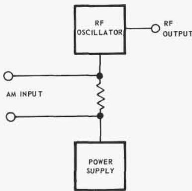
Figure 4. Amplitude Modulation
