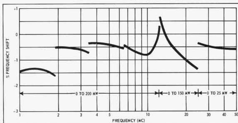
Figure 10. Typical Frequency Shift - No Load to Specified Output and Worst Mismatch
