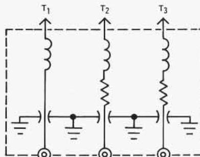
Figure 3. Equivalent Filter Circuit
