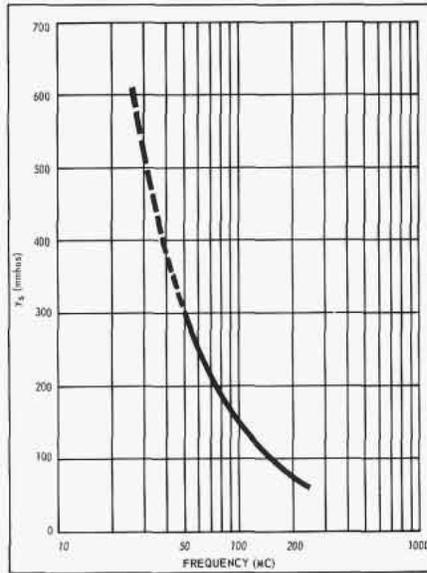
Figure 7.  $y_s$  vs. Frequency Correction — Above 50 mc
