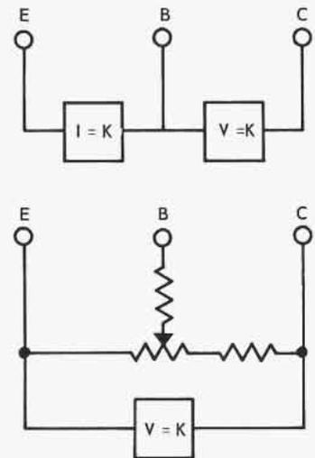
Figure 4. Recommended Bias Supply Configurations
