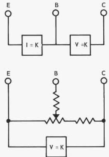
Figure 4. Recommended Bias Supply Configurations
