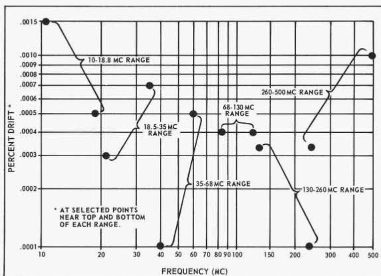
Figure 3. Typical Frequency Drift — For 5 Minutes After 4-hour Warmup
