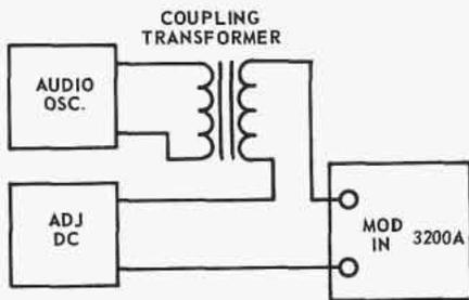
Figure 5. Setup for Obtaining Modulation in Excess of 40%
