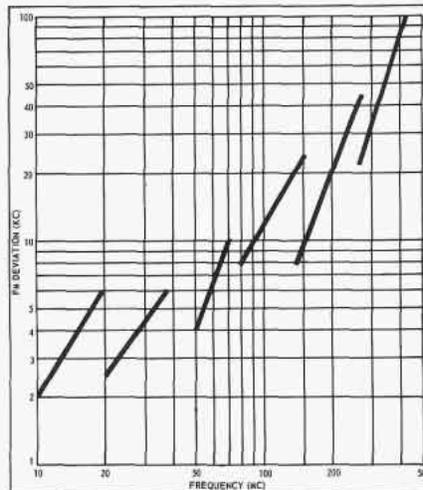
Figure 6. Typical FM Deviation for Fixed Audio Input Level
