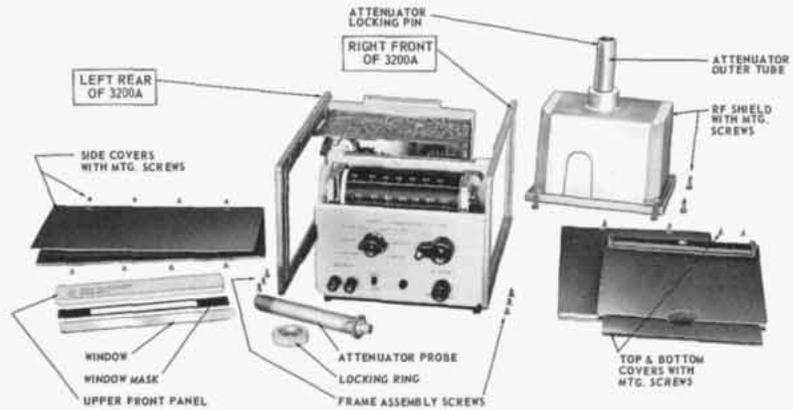
Figure 13. 3200A — Disassembled
