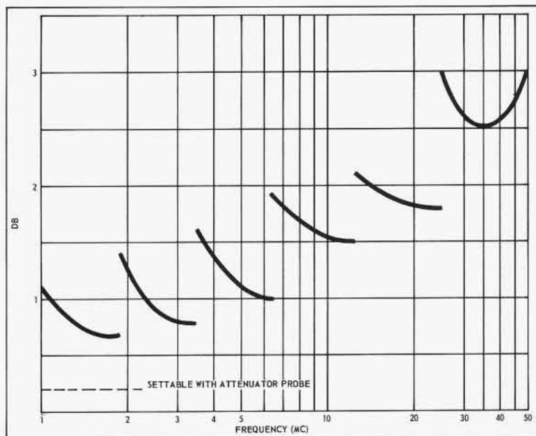
Figure 9. Typical Settability Using Electrical Vernier
