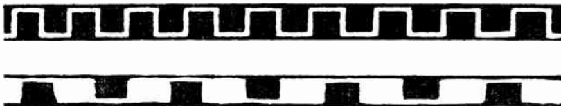
Fig. 7. Actual-size reproductions of comb-pattern metallized paper. The black portions of the pattern are the metallized part of the paper strip. Upper pattern is used where only one thickness of paper is needed between the electrodes, while lower pattern is for higher-voltage capacitors requiring two thicknesses of insulating paper.
