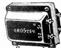
Fig. 4—Audio Transformer as Used in Older Crosley Sets.
