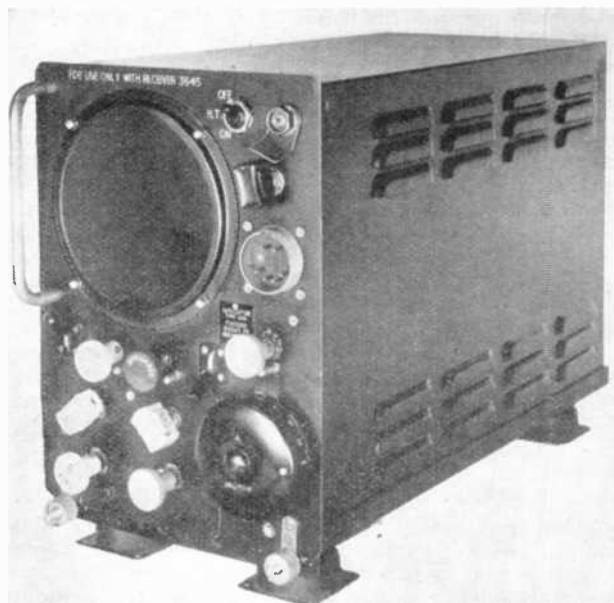
An early type of radar unit. This is the GEE Mk. II Indicator which went into production in 1942 and which has continued in service up to the present time. Reproduced by courtesy of Messrs. A. C. Cossor, Ltd.
