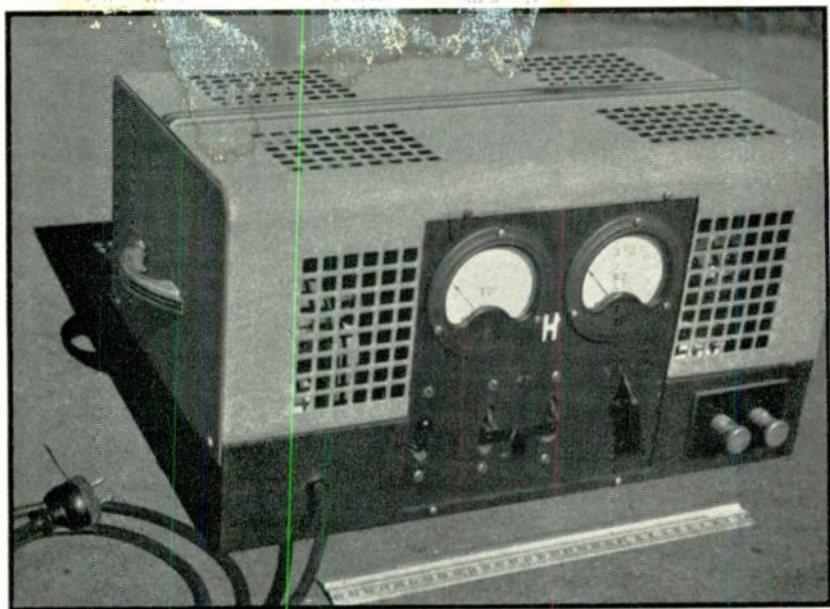
High-current gas-type full-wave rectifier assembled in well-ventilated metal cabinet, and rated to deliver up to 9 amp at 90 v. D-C output terminals are at right on panel. The meters are connected to read output voltage and current. Total weight is 39 lb.—much less than an M-G set having equal capacity.
