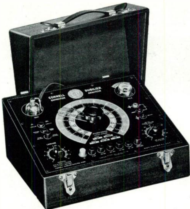
Fig. 3. Capacitor analyzer using a capacity bridge and adjustable d-c power supply.
