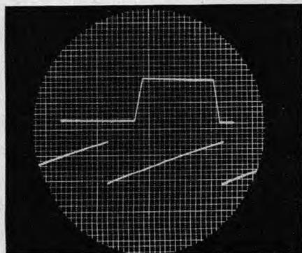
Figure 9. The 1-volt calibration standard, a clipped sinewave, is shown with a sawtooth waveform which has been set at a 1-volt peak amplitude externally by using the scale calibration.
