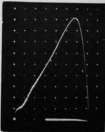
Figure 2. Matrix of dots for voltage calibration along X and Y axes
