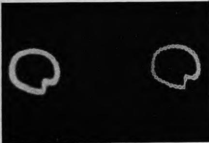
Figure 4. Integrated polar coordinate display of the averaged thread tension on a loom obtained by multiple exposures
