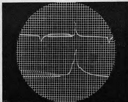
Figure 8. The field surrounding a fluorescent lamp is shown without expansion on the upper trace. A portion of the same signal is shown on the lower trace, expanded to resolve the detail
