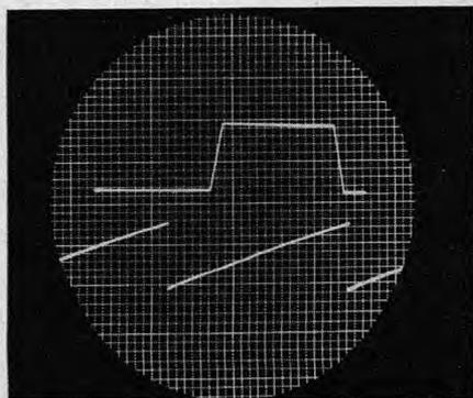
Figure 9. The 1-volt calibration standard, a clipped sinewave, is shown with a sawtooth waveform which has been set at a 1-volt peak amplitude externally by using the scale calibration.
