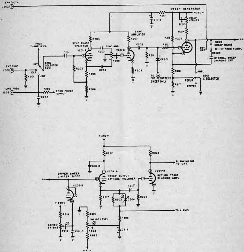
Figure 3. Sync and sweep circuits, simplified schematic
