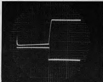
Figure 5. Input (lower trace) and output (upper trace) of an amplifier circuit using the common sweep of the new Type 322. The frequency is 1 KC. Note how the loss in rise time may be conveniently measured
