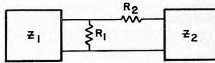
Figure 5. Resistor-matching network for low impedances.
