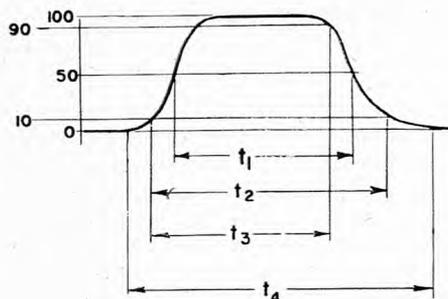
Figure 2. Various definitions of pulse width.
