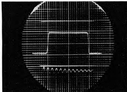
Figure 8. Pulse displayed with time-calibration wave train and amplitude-lines.
