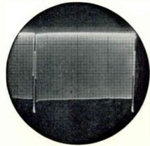
Figure A-3. Output of first sync clipper with narrow-band transformer properly adjusted.
