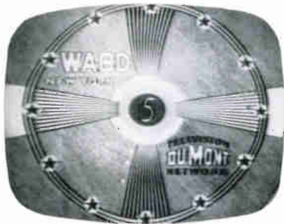
Figure T-2. Slight picture smear accompanied by heavy streaking noise visible at the vertical wedges of the test pattern. This condition was caused by a defective component in the grid circuit of the video amplifier.
