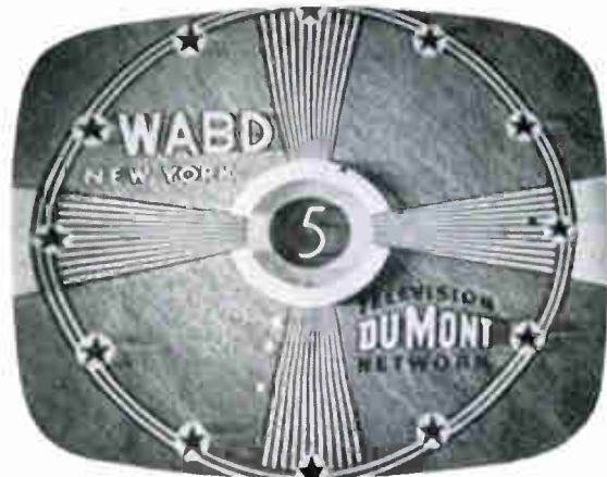
Figure T-1. The test pattern shown above exhibits the effects of trailing blacks and whites upon the picture. Although this condition can be the result of an improper video i-f alignment, the above was due to a defective component in the video amplifier.
