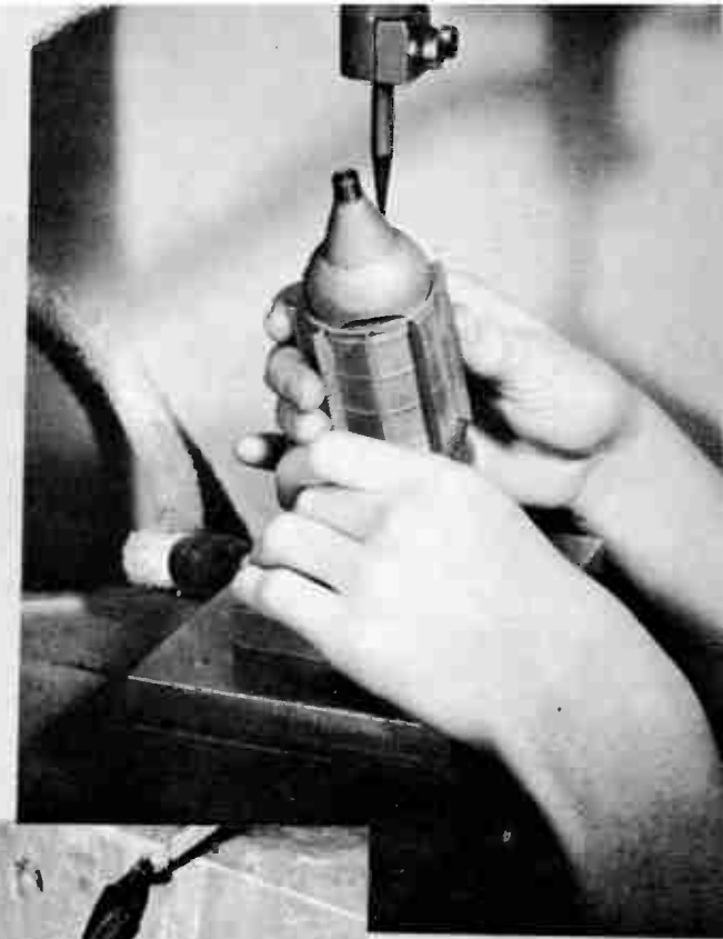
The assembly is rapidly nearing completion as it is shown here with hat and cone welded to the plate
