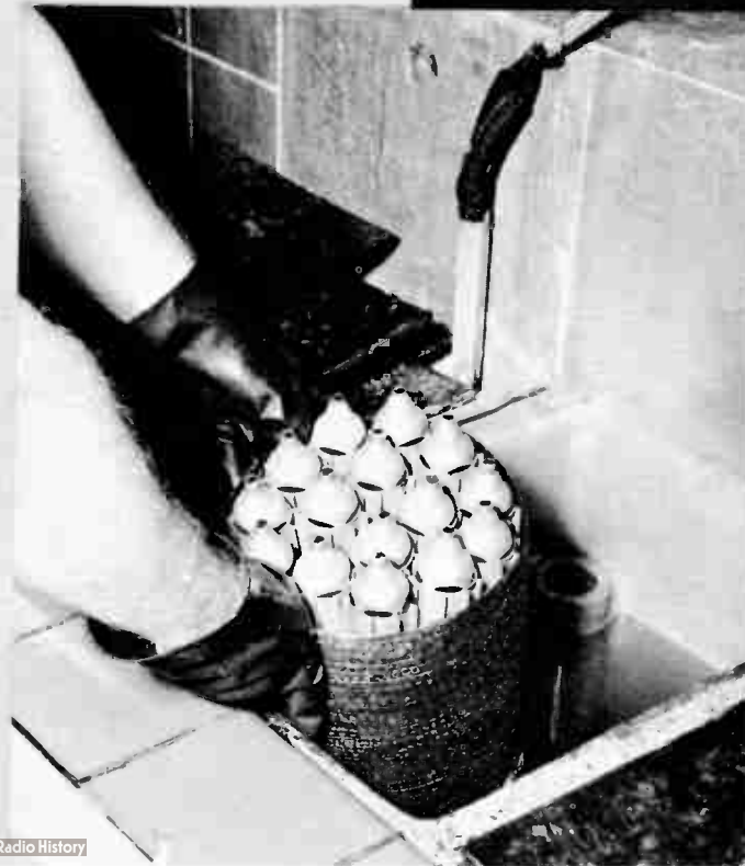
In the Chemical department the plates with hats and cones are placed in a chemical cleaning solution, which rids the assembly of copper spots acquired in the spot-welding operation
