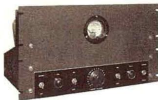
Fig. 2—Front-panel View of Thyatron Rectifier Power Supply
