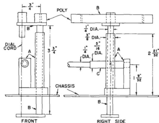
Fig. 7. Guillotine Tuner Dimensions
