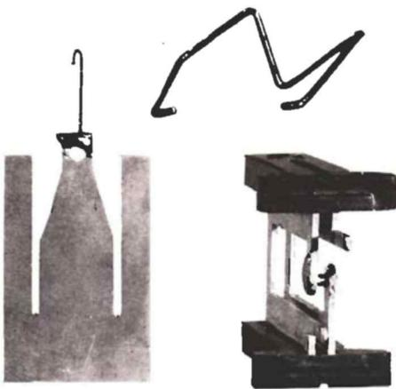
Fig. 3. Detail View of Guillotine Coil
