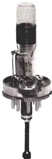
Fig. 3. Detail View of Oscillator Plate Coil.
