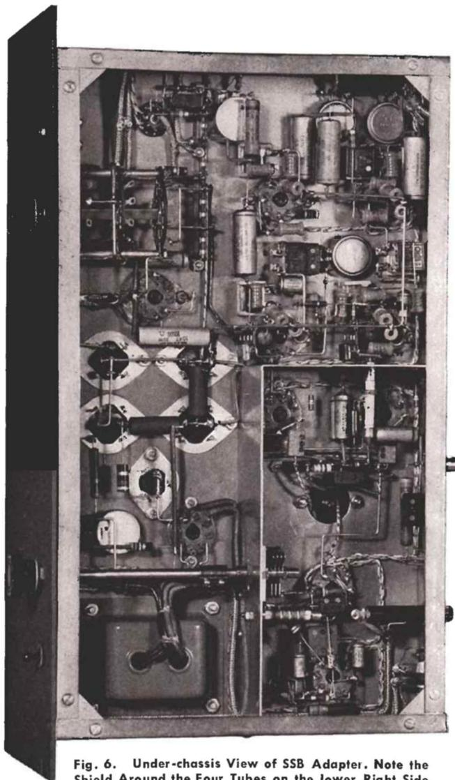
Fig. 6. Under-chassis View of SSB Adapter. Note the Shield Around the Four Tubes on the lower Right Side
