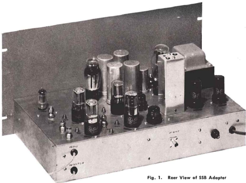
Fig. 1. Rear View of SSB Adapter
