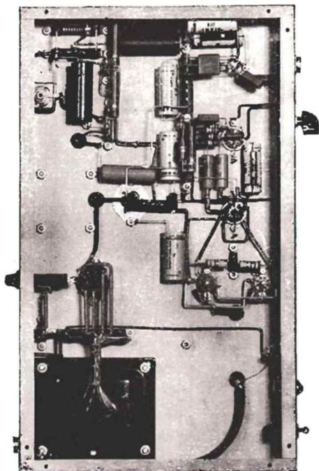
Fig. 4. Under-chassis View of the Restricted-range Speech Amplifier
