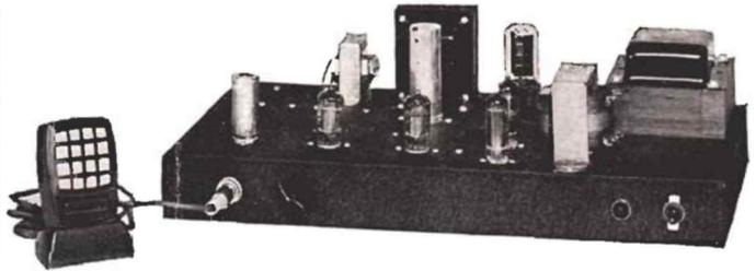
Fig. 1. Front View of the Restricted-range Speech Amplifier
