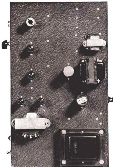
Fig. 5. Top View of the Restricted-range Speech Amplifier
