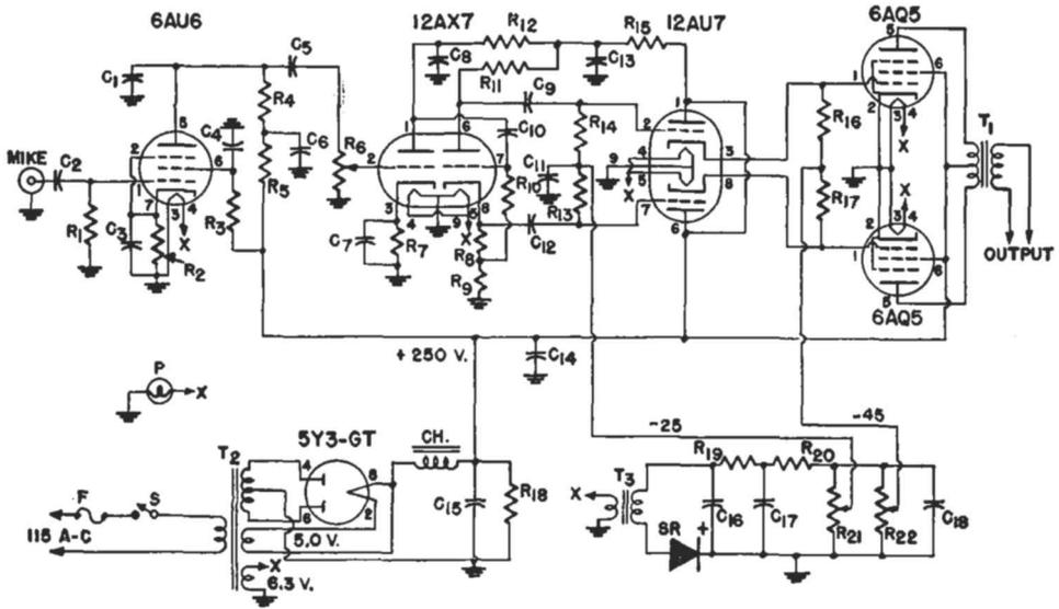
Fig. 2. Circuit Diagram of the Restricted-range Speech Amplifier
