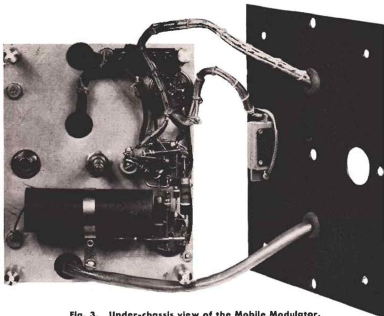
Fig. 3. Under-chassis view of the Mobile Modulator.
