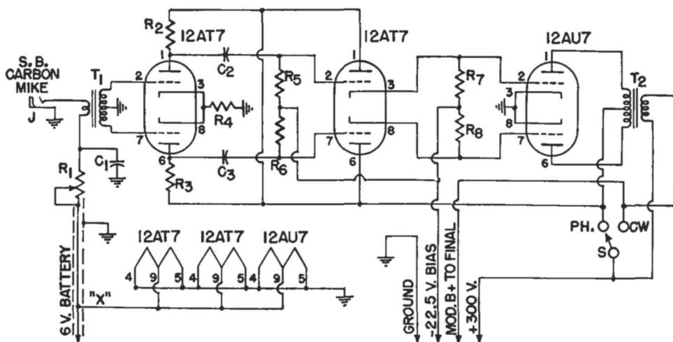
Fig. 2. Circuit diagram of the Mobile Modulator.
