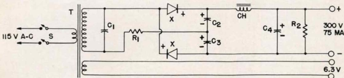
Fig. 6. Circuit diagram of the Utility Power Supply.
