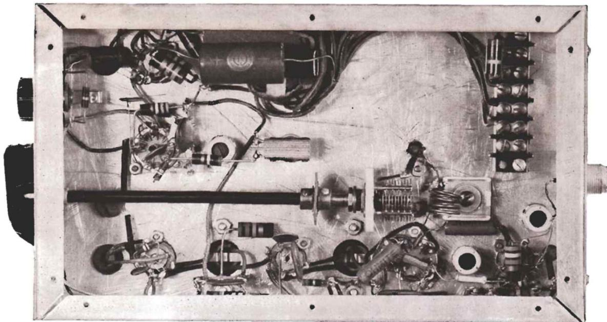
Fig. 3. Underchassis view of the 6-Meter CD Receiver
