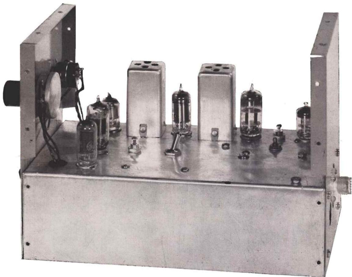
Fig. 1. Side view of the 6-Meter CD Receiver
