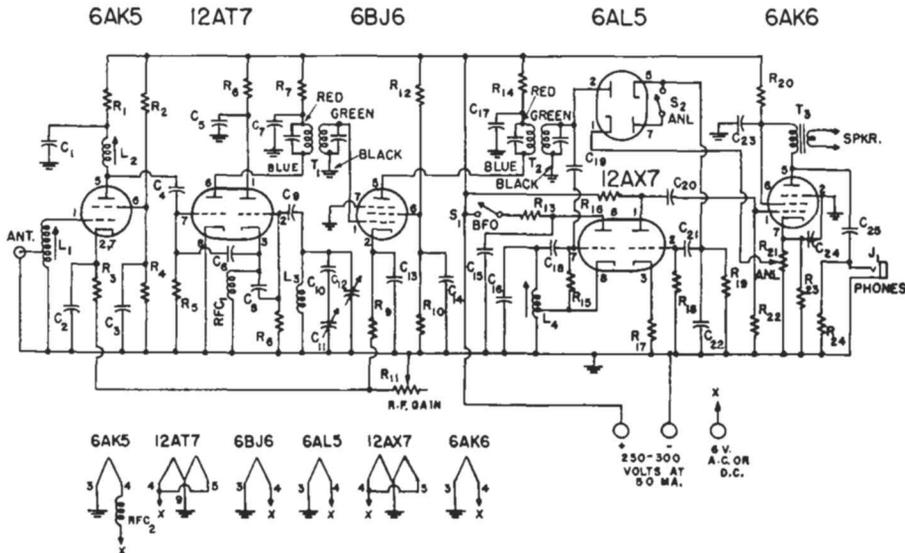
Fig. 2. Circuit Diagram of the 6-Meter CD Receiver
