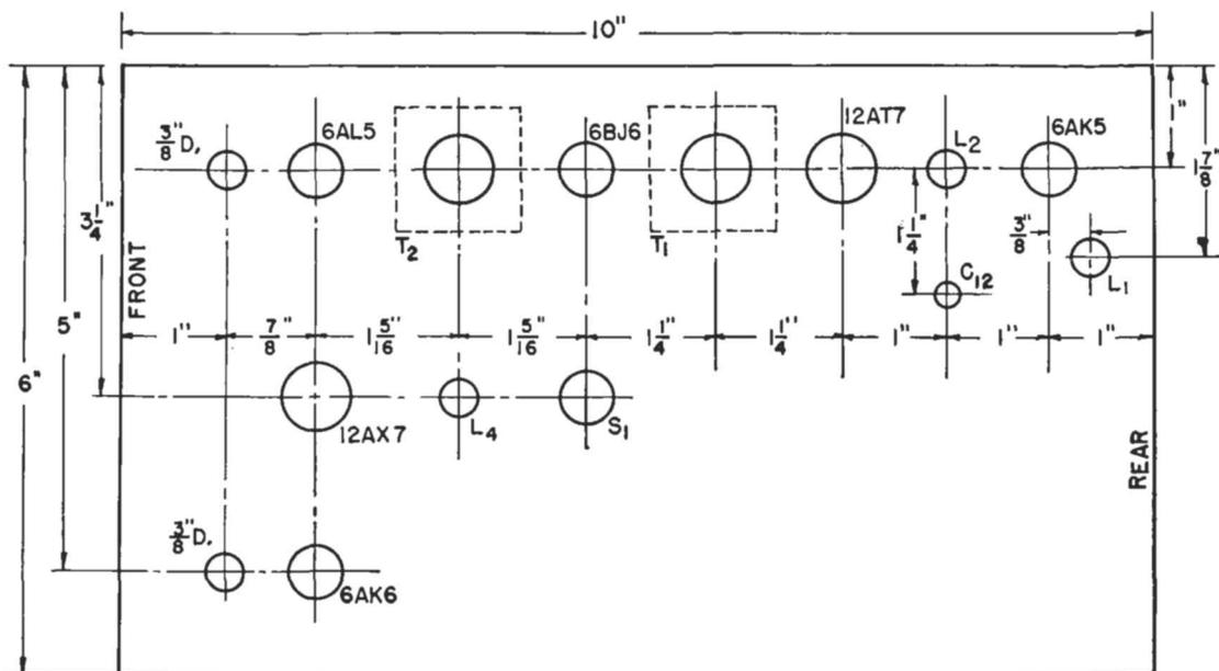
Fig. 5. Chassis layout of 6-Meter CD Receiver
