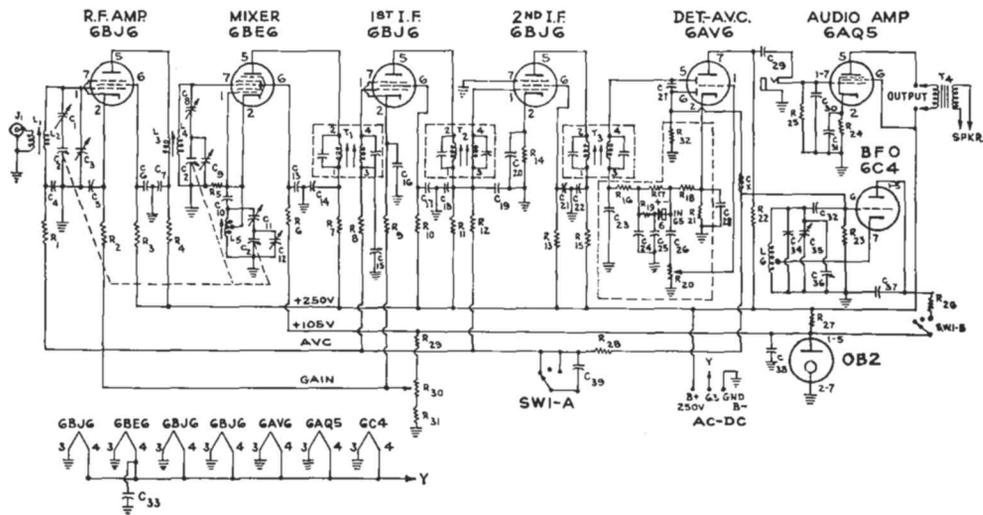
Fig. 2. Circuit diagram of the Mobile-Marine Receiver.
