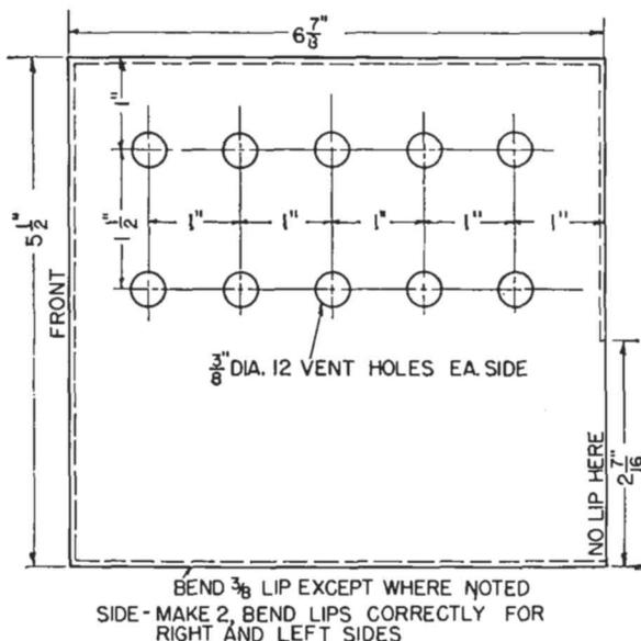
Fig. 8. Side panel layout for Mobile-Marine Receiver.
