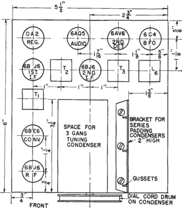
Fig. 5. Chassis layout of the Mobile-Marine Receiver.
