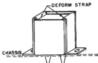
Measure the distance across the capacitor inside the beaded edges, and fabricate, from soft aluminum
