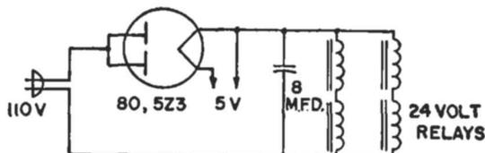
output voltage of this supply with one 8-microfarad condenser for filter is about 50 volts or sufficient to operate 2 relays in series, but the current available is sufficient to operate two or three strings of relays.
