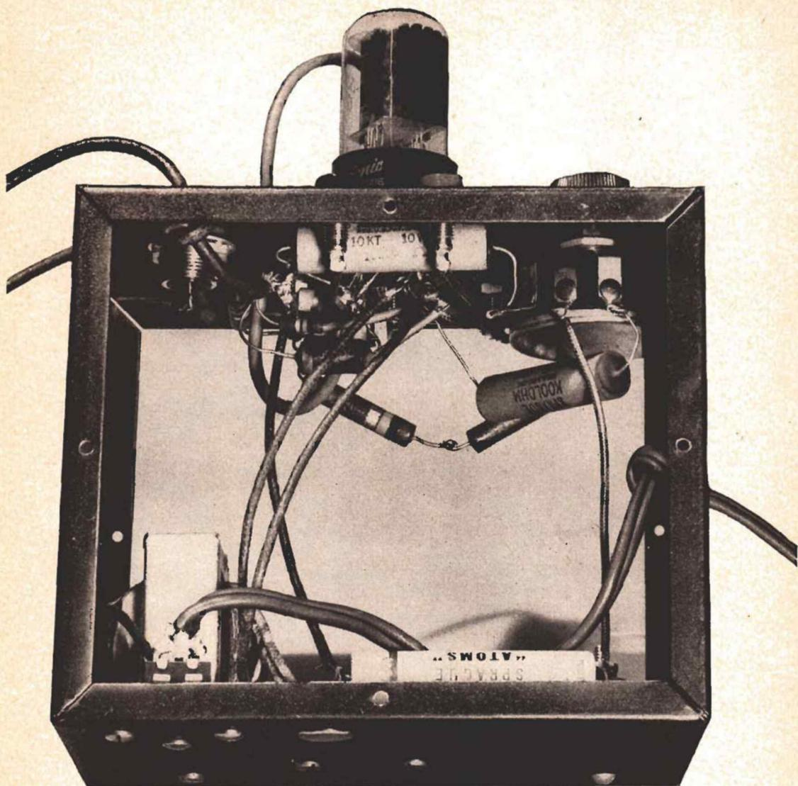
signal generator, an RF voltage of 4 volts read 3.8 volts with the Adapter-multi-meter combination. Above 10 megacycles the sensitivity fell off and the Adapter no longer gave an accurate reading. However, the presence of RF on the coil of a grid dip oscillator was still indicated by the Adapter up to 250 megacycles.
