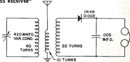
layer of plastic electrician's or scotch tape for insulation. The selectivity of this circuit is also fairly good because the 1N48 crystal diode does not load the tuned circuit heavily.
