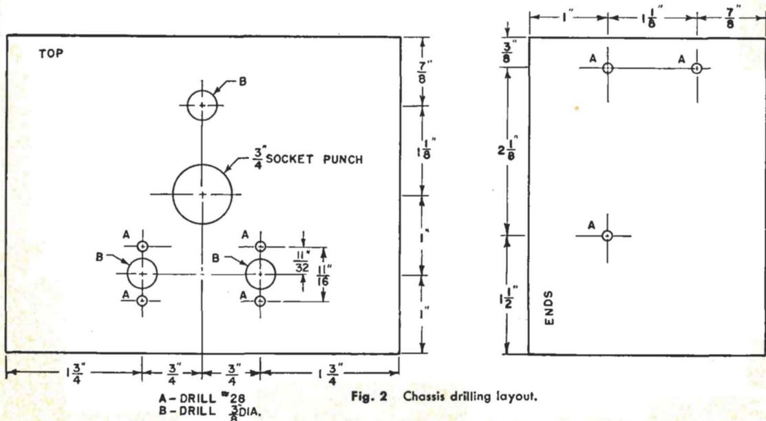
Fig. 2 Chassis drilling layout.
