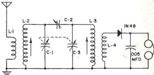
loopsticks for maximum volume as well as for proper tracking of the tuned circuits when several stations are to be received. The coupling condenser,  $C_2$ , is a 3-30-mmfd compression type trimmer. It is adjusted for maximum volume on local stations or maximum selectivity on distant stations. Imagine a crystal receiver with a selectivity control!!
