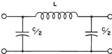
the filter must be terminated by the same impedance. Ideally, too, the filter elements should be perfect reactances. Practically speaking, the characteristic impedance varies throughout the pass-band of the filter. Of course, the filter elements do have loss (they are not perfect reactances) so that other considerations
