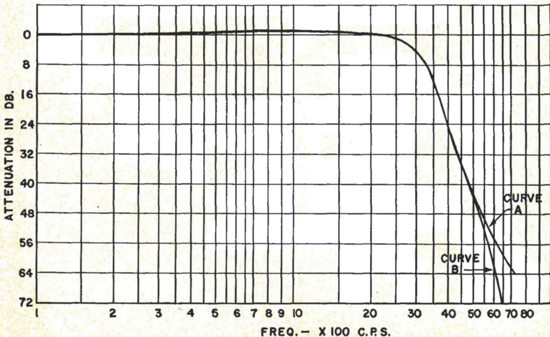
Fig. 6 Response curves with and without coils oriented.
